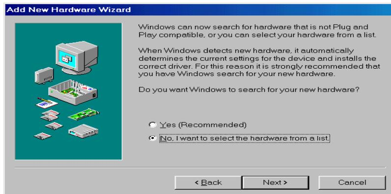
5. The first time the software is installed, select **Other Devices** from the following screen. Once the device database is modified, **Motion** will be listed in the hardware types list. Select the motion type for future device additions.
