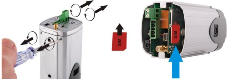
Insert the SIM card into the holder with the metal contacts facing to the SIM connector side. Ensure that the 'cut-off' corner is at the bottom right as in figure above. After the SIM card is inserted attach the panel to its previous position.
