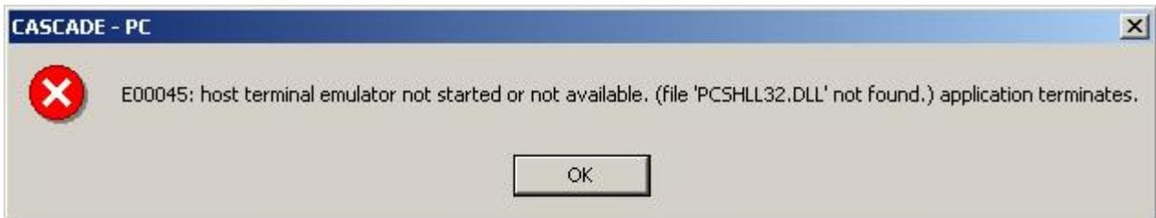
In this case you will have to start the terminal emulation and then CASCADE-PC. Should the message be repeated, re-boot the PC and start the applications in the required order.
