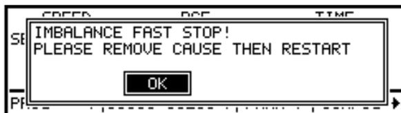
Run cannot be continued (imbalance > cut-off limit). Run is terminated with max. deceleration.
