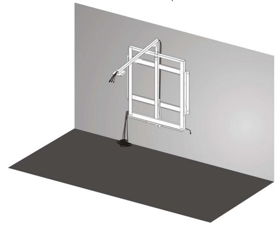
**10.** Install the Interactive Board on the stand and make sure the upper attachment point matches the attachment point of the IB.
