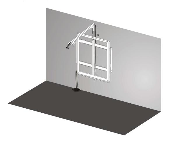
**9.** Place the USB/RS-232 cable in the stand. Make sure to leave the RS-232 interface on the IB side and the USB to connect on the computer.
