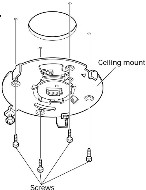
1. Make a hole (90 mm dia.) in the ceiling for passing through the connection cables.
