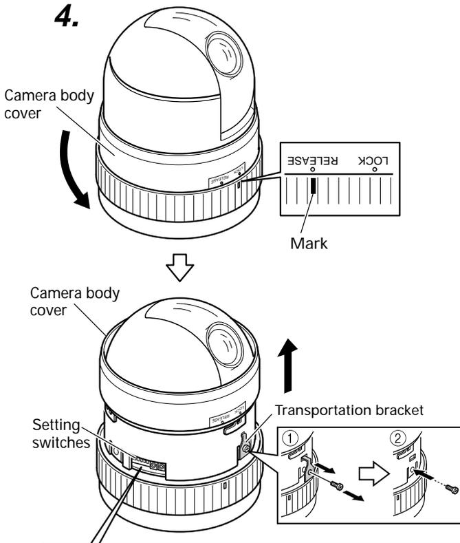
**4.** Turn the camera body cover to anti clockwise to set the word "RELEASE" on the camera body cover over the mark, then pull the camera body cover upward. Transportation bracket is mounted when it is shipped from the factory. Make sure to remove it before installation.
