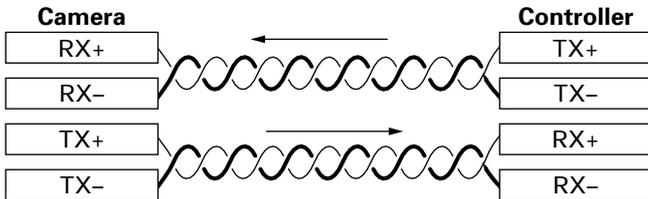
Four wires must be connected.
