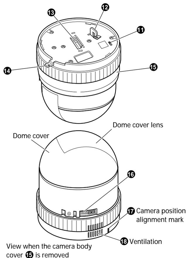
View when the camera body cover 15 is removed
