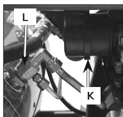
**Air Intake Filter (K):** This filter is designed to clean air coming into the pump. This filter must always be clean and ventilation openings free from obstructions. See "Maintenance".
