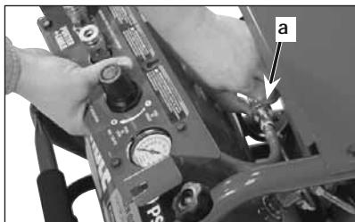
3. Connect air hose (sold separately) to quick connect plug (b) and quick connect (a). The console can then be brought closer to the work site to rest on the console brackets (d) or be temporarily mounted using the mounting hole (c).
