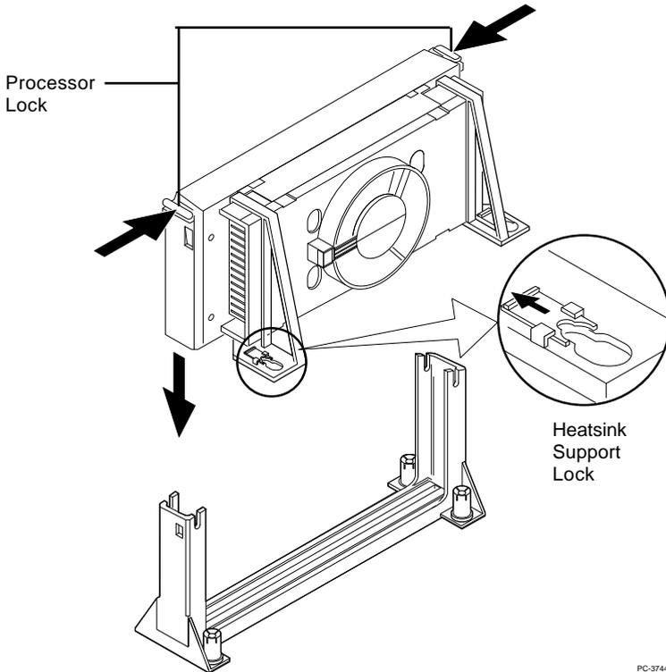
**Step 6:** Insert the Processor like inserting a PCI or an ISA card.
