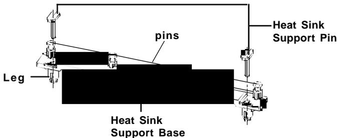
Push the Heat Sink Support Base onto the mainboard, until you hear a click sound. Check for a perfect fit.
