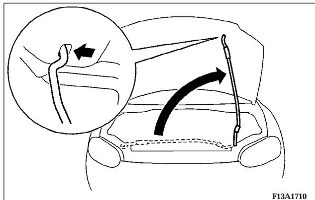
Support the engine hood with the hood prop by inserting the hood prop securely in the opening in the hood marked with an arrow.
