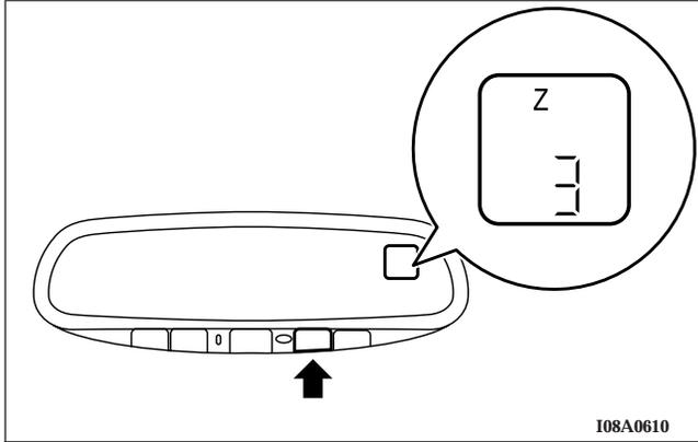
6. If you press the display switch more than 12 seconds, you can recalibrate compass variance. →186
