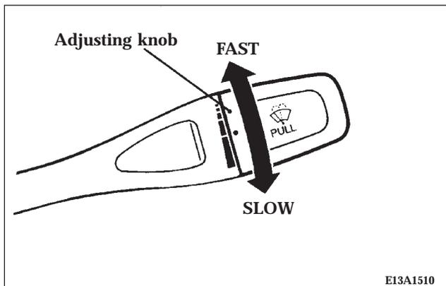
Use the intermittent feature when weather conditions make a single wiping cycle, with a pause between cycles, desirable.
