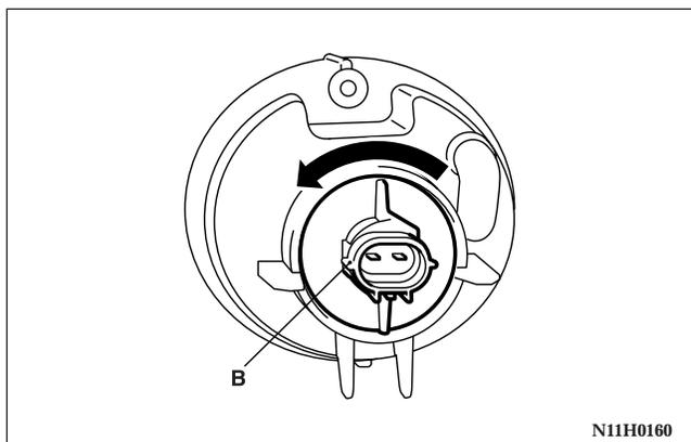
3. Remove the entire socket and bulb assembly (B) by turning it counterclockwise.
