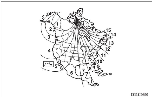
3. Press the display switch until the new zone number appears in the display. After 5 seconds of inactivity, the original item (Outside temperature/Compass) displayed again.
