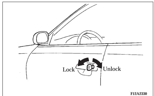
Rotate the key toward the front of the vehicle to lock the door. After checking that the door is locked, turn the key back to the center and remove it from the lock cylinder.
