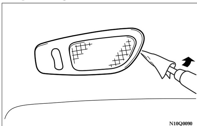
Insert the tip of a flat blade screwdriver at the edge of the lens, pry gently to remove the lens, and then remove the bulb from the light holder.
