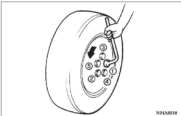
9. Remove the wheel nuts with the wheel nut wrench, then take the wheel off.
