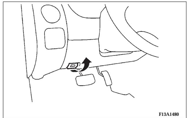
The engine hood release lever (located under the instrument panel near the driver's door) is used to unlock the engine hood. Pull the lever toward you to release the engine hood latch.
