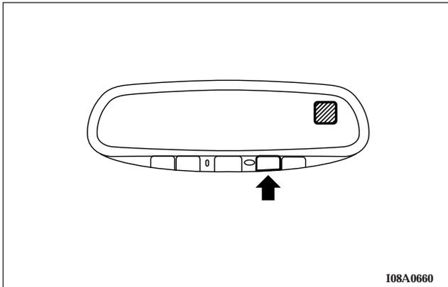
3. If you press the display switch more than 3 seconds, less than 6 seconds, you can alternate the temperature reading between Fahrenheit and Celsius. → P. 182.
