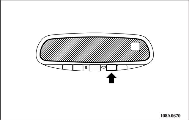
5. If you press the display switch more than 9 seconds, less than 12 seconds, you can adjust for compass variance. →183
