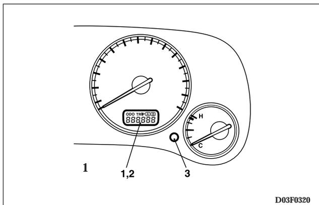
When the ignition switch is turned to the “ON” position, an “ODO” or “TRIP” indication is given. Every time the reset button (3) is pressed lightly (less than one second), the indicators will change from “ODO” to “Trip A” to “Trip B”.
