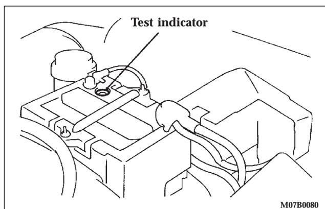
The condition of the battery is very important for quick starting and proper functioning of the vehicle's electrical system. Check the battery at regular intervals. To determine the battery charge, check the battery test indicator on top of the battery.
