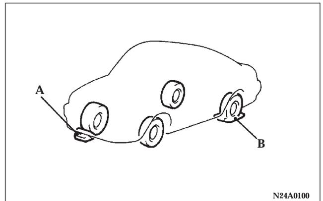
4. Apply a chock or block (A) at the tire diagonally opposite the tire (B) to be changed.
