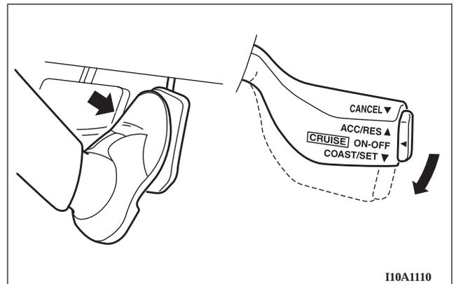
Press the brake pedal (which disengages the cruise/speed control), then pull the cruise/speed control lever down momentarily to set a new desired cruise speed.
