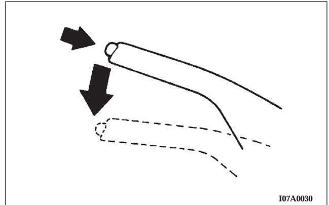
When parking on a hill, it is important to set the parking brake before placing the gear selector in Park, otherwise the load on the transmission locking mechanism may make it difficult to move the selector out of Park. As an added precaution, turn the front wheels toward the curb on a downhill grade and away from the curb on an uphill grade.
