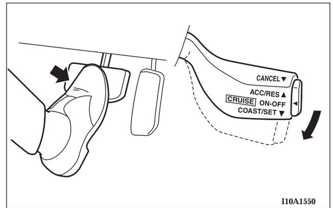
Press the accelerator pedal to reach your desired speed. Pull the cruise/speed control lever down for a moment, then release it.
