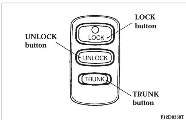
Press the keyless transmitter button(s), and all doors will be locked or unlocked as desired. The PANIC button can also help you signal for attention.
