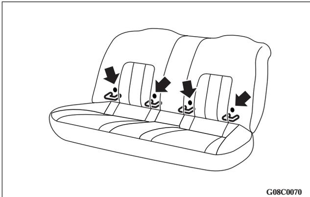
Your vehicle's rear seat is fitted with lower anchorages for attaching a new child restraint system that complies with Federal Motor Vehicle Safety Standard 213.
