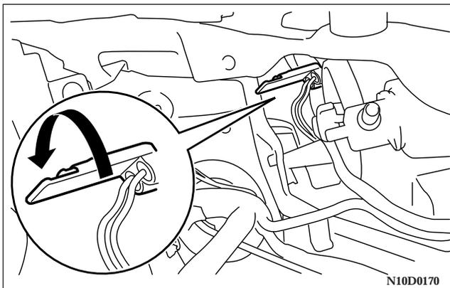
Turn the light socket counterclockwise and pull it out and remove the light bulb.
