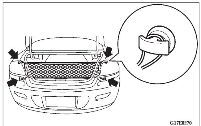
Attach the net to hooks according to the illustration. Keep the net stored in the trunk so it can be used at any time.
