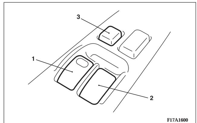
The main driver switch can be used to operate both door windows.
