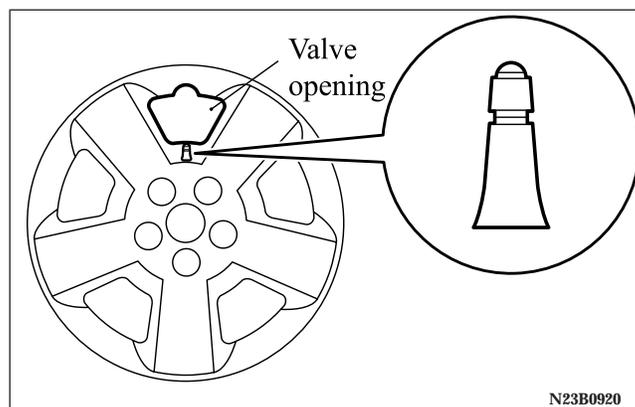
Align the air valve with the valve opening provided on the wheel cover.
