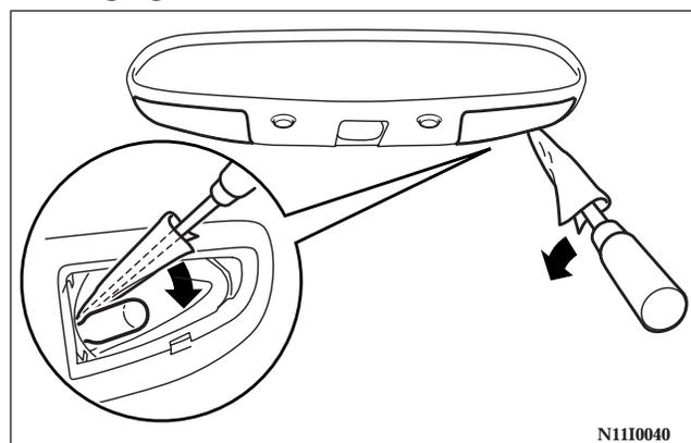
Insert a straight blade screwdriver into the notch of the light assembly and pry gently to remove the lens. Remove the light bulb from the light holder.
