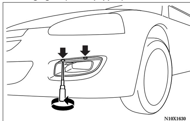
1. Insert a screwdriver as shown in the illustration and remove the screws.
