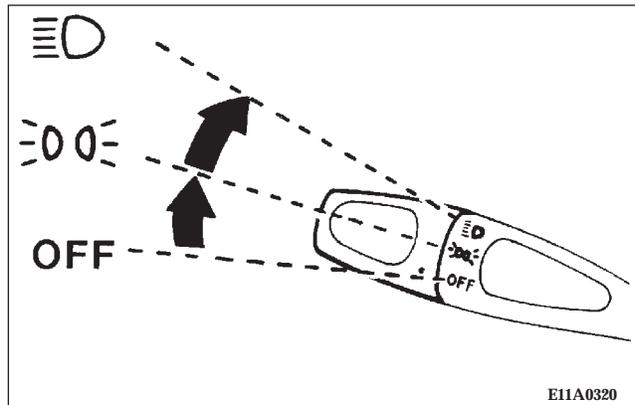
Rotate the switch to operate the lights.
