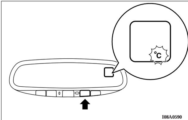
Press the display switch above 3 seconds, less than 6 seconds until the display blinks °F and °C.
