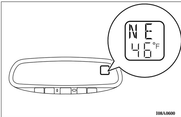
When the ignition key is in the “ACC” or “ON” position, the vehicle’s current directional heading (N, NE, E, SE, S, SW, W and NW) will be displayed.
