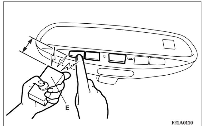
4. Using both hands, press the hand held transmitter button and the desired universal transceiver button. Do not release the buttons until step 5 has been completed.
