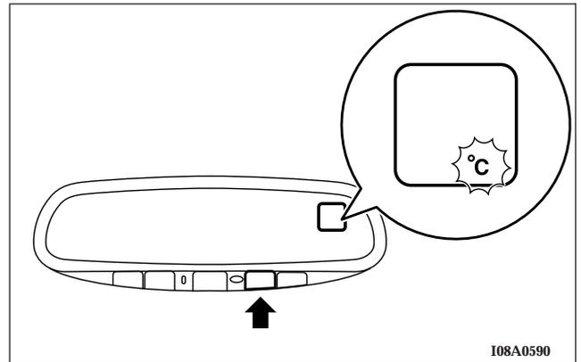
4. If you press the display switch more than 6 seconds, less than 9 seconds, you can turn on/off the automatic anti-glare. → 177
