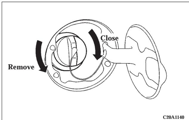
Remove the fuel tank filler tube cap slowly by turning it counterclockwise.
