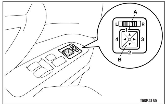
The outside rearview mirrors can be adjusted when the ignition key is in the “ON” or “ACC” position.
