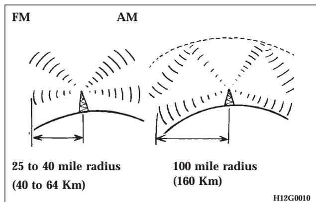
A vehicle is not an ideal place to listen to the radio, because the vehicle moves, and reception conditions are constantly changing. Buildings, terrain, signal distance and noise from other vehicles are all working against good reception.
