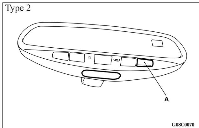
Push the light switch (A) to turn on the light, and push the light switch again to turn them off.
