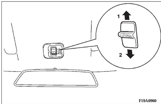
The sunroof can be opened and closed with the ignition key in the "ON" position.
