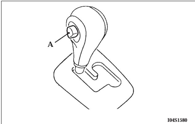
In the main gate, the selector lever has 4 positions and is equipped with a lock button (A) to prevent inadvertent selection of the wrong gear.
