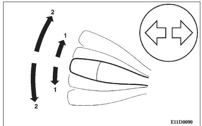
For changing lanes, or when making a gradual turn, the lever may be held in the “lane change” position (1). It will return to the neutral position when released. The fully engaged position (2) is for use when making a normal turn. The lever will return automatically upon completion of the turn.
