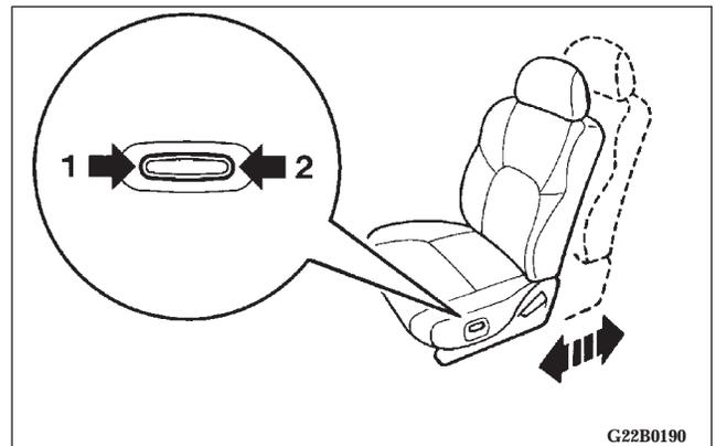
Push the switch to adjust the seat forward or backward to the desired position. Release the switch, and the seat will lock at that position.
