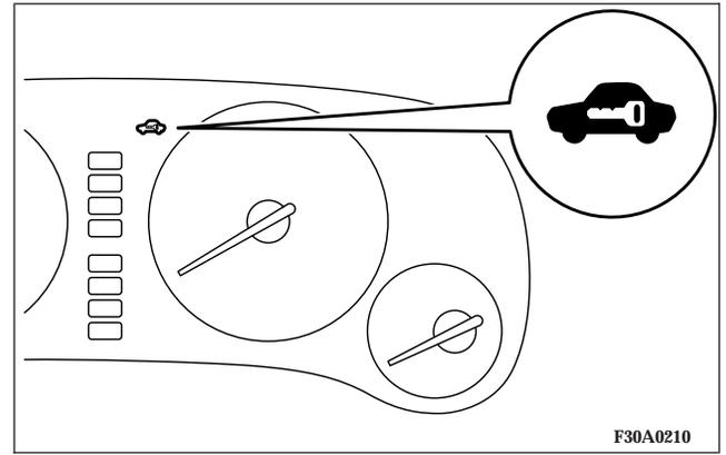
After completion of the steps above, the theft-alarm indicator (located in the instrument cluster) will illuminate for approximately 20 seconds and then go out, indicating that the system is armed.
