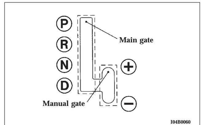
The transaxle has 4 forward gears and 1 reverse gear. The individual gears are selected automatically, depending on the position of the gear selector lever, the speed of the vehicle, and the position of the accelerator pedal. The selector lever has 2 "gates": the main gate and the manual gate.
