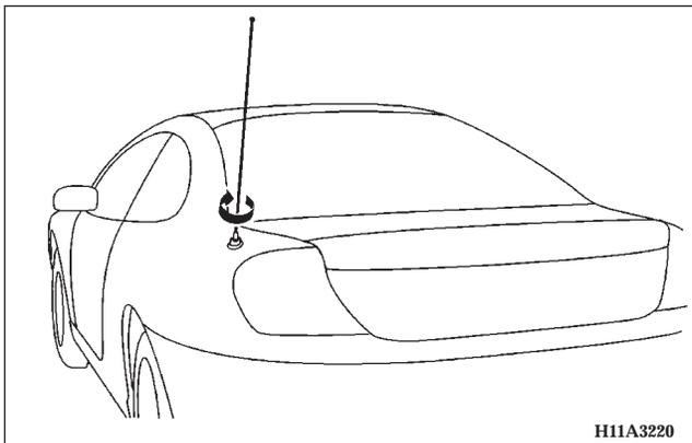
To remove the whip antenna, turn it counterclockwise.
