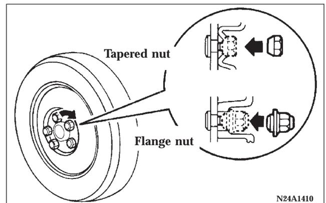
**NOTE:** Clear out any mud, etc. on the hub surface, hub bolts or in the installation holes in the wheel.
