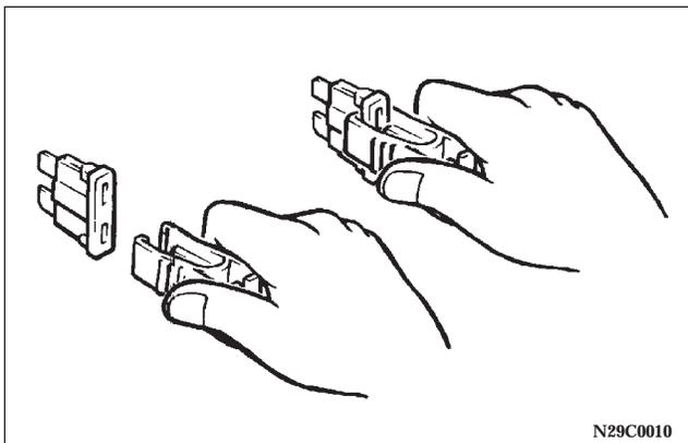
5. Insert a new fuse of the same capacity securely into the fuse block location.
