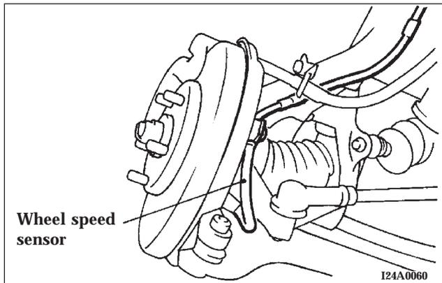
3. After driving on snow or icy roads, remove any snow and ice that may have adhered to the wheel areas. When doing this be careful not to damage the wheel speed sensors and cables located at each wheel on vehicles equipped with an anti-lock braking system.
