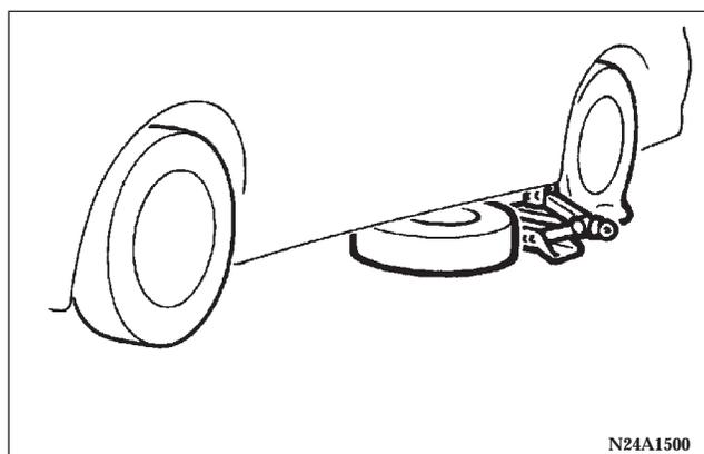
**NOTE:** Place the spare wheel under the vehicle body near the jack; this helps to minimize danger should the jack slip out of position.
