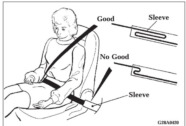
The lap belt portion of the front UNIBELT has a sleeve inside which the belt is folded back over itself in a loop. This allows the belt to help absorb the energy of a collision through a controlled release of the loop. In the event that the loop inside the sleeve has come loose, replace the entire seat belt assembly.
