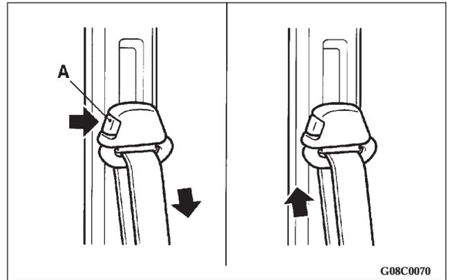
The seat belt shoulder anchor height can be adjusted for greater comfort.
