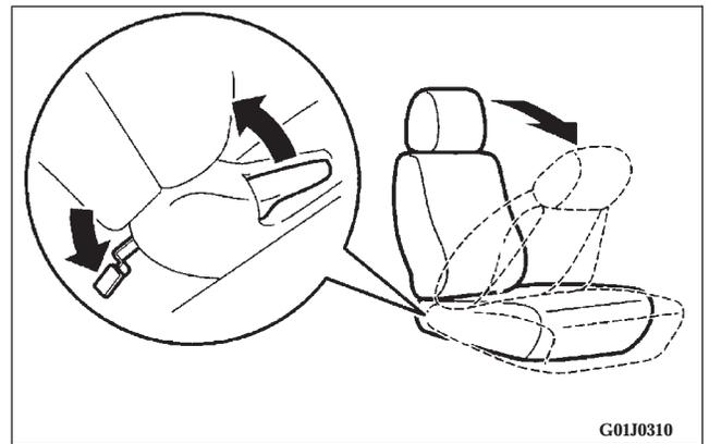
To permit rear seat entry or exit, the front seatback will fold down and the seat will move forward when the seatback lock lever is pulled up or when the pedal in back of the front passenger seat is depressed. To return the seat, push the seatback backward until there is a "click" and the seat locks in position.
