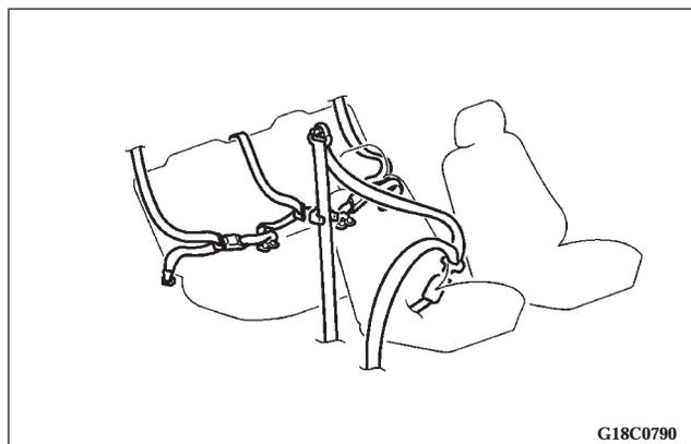
The UNIBELT at the rear seat positions, and at the front passenger seat, can be converted from normal Emergency Locking retractor (ELR) mode, to Automatic Locking Retractor (ALR) mode. It must be converted to the ALR mode when installing a child restraint system.
