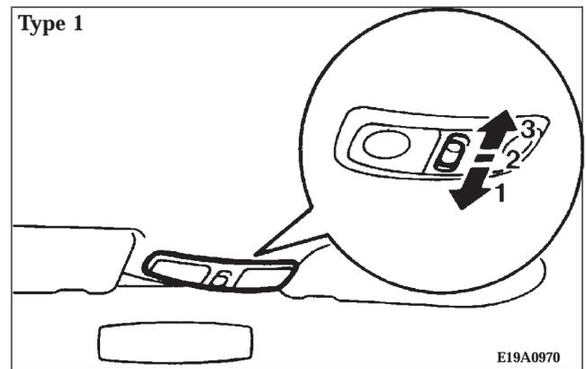
The dome/reading light can be operated by moving the switch as follows:
