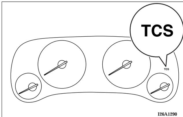
When the ignition key is turned to “ON”, the warning light illuminate and go out after a few seconds.
