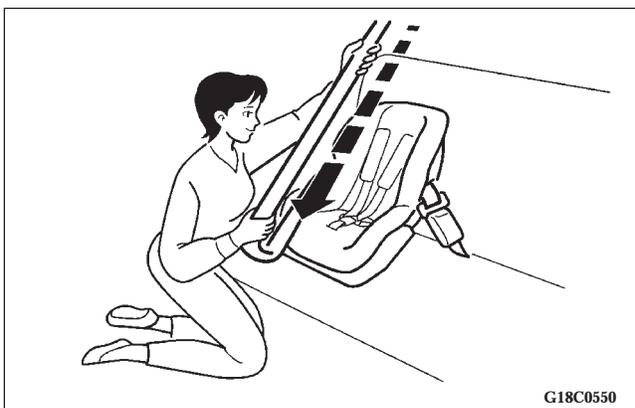
3. To activate the ALR mode, slowly pull the shoulder part of the belt all the way out until it stops, then let the belt feed back into the retractor.
