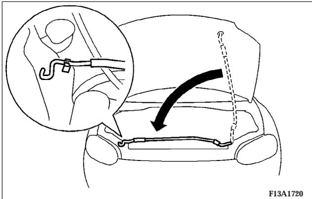
To close, unlatch the hood prop from the engine hood and place the hood prop in its retainer. Slowly lower the engine hood to about 12 inches (30 cm) from the closed position, then release it. The hood should latch from its own weight.
