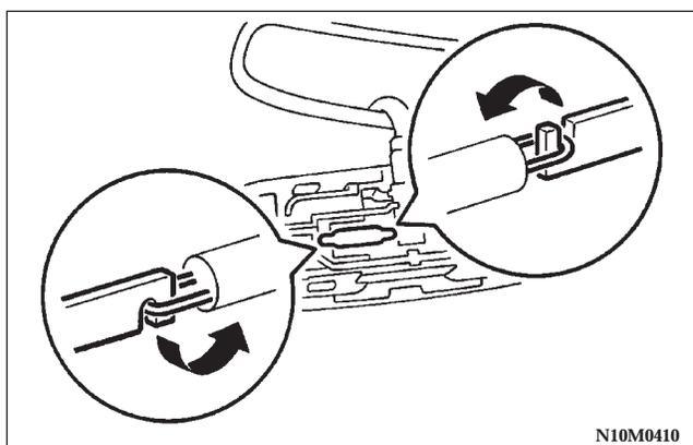
2. Remove the light bulb from the light holder.
