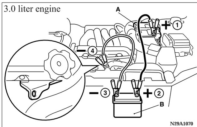
5. Connect one end of one booster cable to the positive (+) terminal of the discharged battery (A), and the other end to the positive (+) terminal of the booster battery (B).
