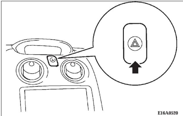
Press the flasher switch and the front and rear turn signals will flash intermittently, as the hazard warning lights. This is an emergency warning system and is not intended for use when the vehicle is in motion.
