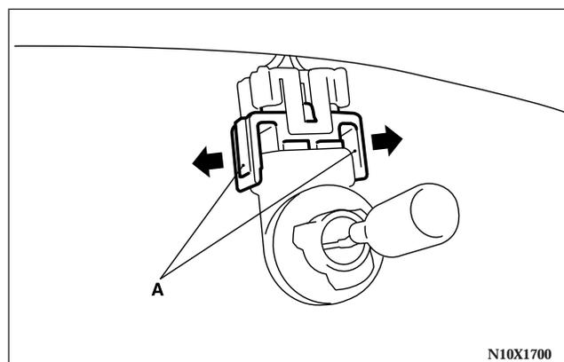
3. Pull both clips (A) away from the center as shown and remove the bulb from the socket by pulling out.
