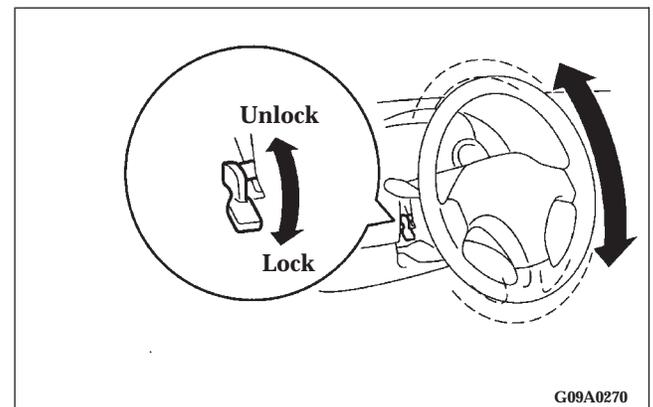
To adjust the steering wheel height, release the tilt lock lever while raising or lowering the steering wheel to the desired height.
