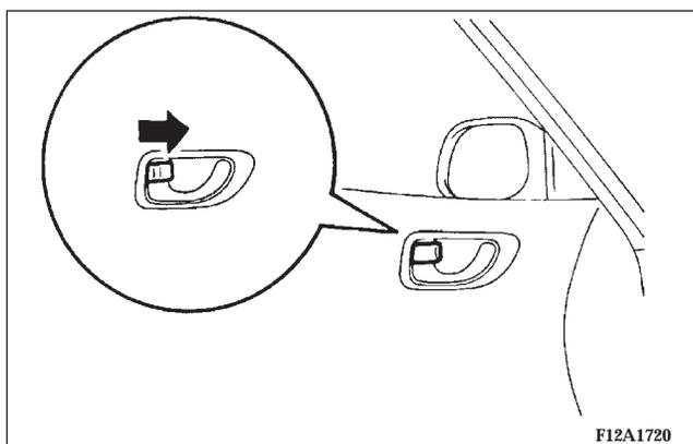
Move the inside lock knob to the locked position (so that the red mark cannot be seen) to lock the door. All doors should be kept locked while driving.
