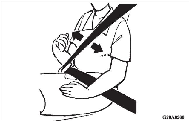
5. The shoulder belt portion will allow regular movement under normal conditions. The belt will lock in the event of an abrupt change in vehicle motion.
