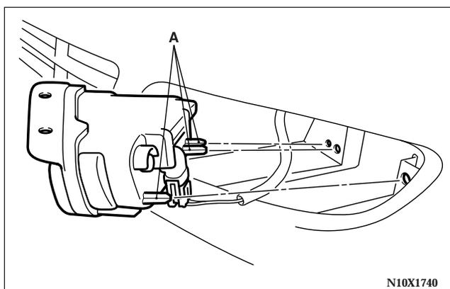
4. When mounting the light unit, align the pins (A) on the light unit with the holes in the body.
