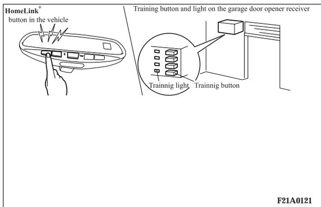
1. Locate the training button on the garage door motor head unit. The exact location and color of the training button may vary by garage door opener manufacturer. If you have difficulty in locating the training button, check your garage door opener manual, or call toll-free for customer assistance at 1-800-355-3515, or on the internet at [www.homelink.jci.com](http://www.homelink.jci.com).
