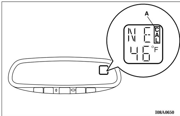
If the display reads “CAL” (A), there may be a strong magnetic field interfering with the compass. In this case, the compass may need calibration.
