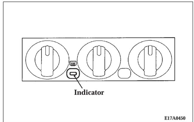
The electric rear window defogger can be operated when the ignition key is in the “ON” position. When the switch is pressed, an indicator in the switch (amber) will illuminate to indicate the electric rear window defogger is on, and electric current will flow through the heating wire on the rear window to clear away fog or frost.
