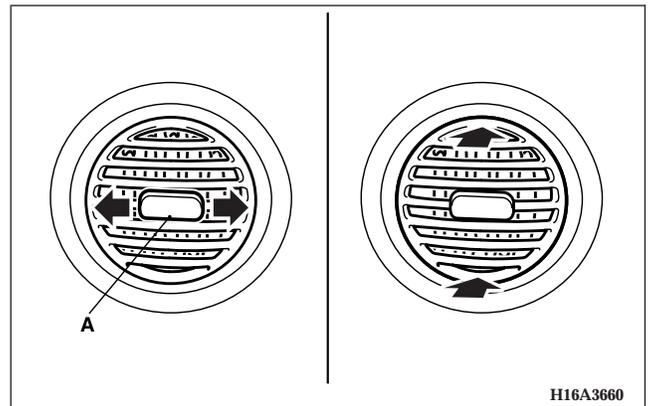
Change the direction of the airflow from side to side by moving the knob (A). Change the vertical direction of the air flow up and down by pushing the top button edge of the vents.
