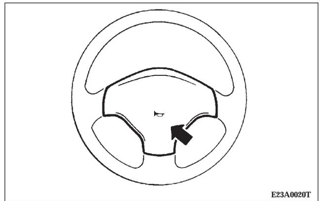
Pressing on or around the
