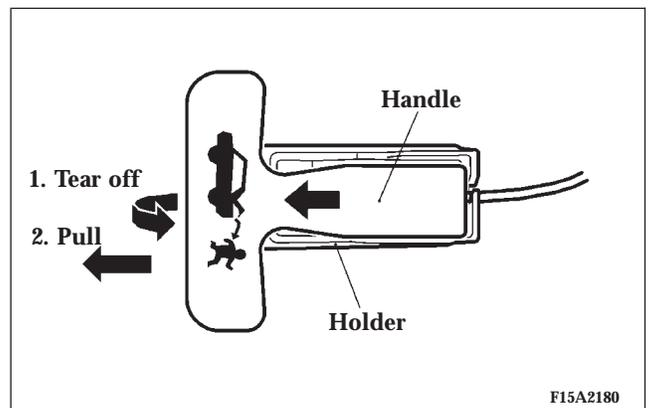
To open the trunk from inside the trunk, tear off the illuminated "T" handle from its holder by pulling in the direction of the arrow (1). Then pull the handle in the direction of the arrow (2). Push up on the trunk to exit.
