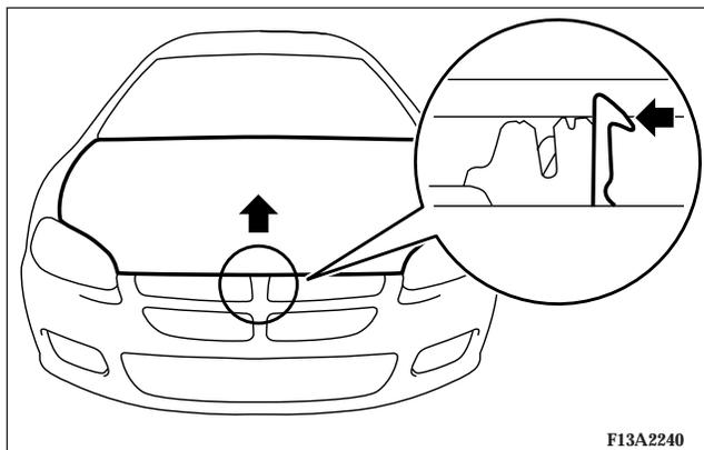
Release the safety lever and lift the engine hood.
