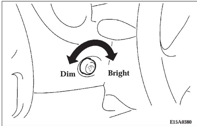
The brightness of the instrument panel lights can be adjusted by turning this knob while the light switch is in the ON “☰” or “☷” position.
