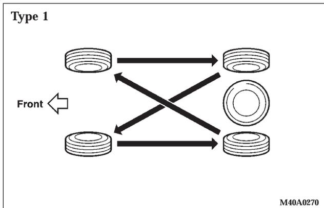
To equalize wear and help extend tire life, the manufacturer recommends that you rotate your tires approximately every 7,500 miles (12,000 km) under normal driving conditions and every 6,000 miles (9,600 km) in severe driving conditions.
