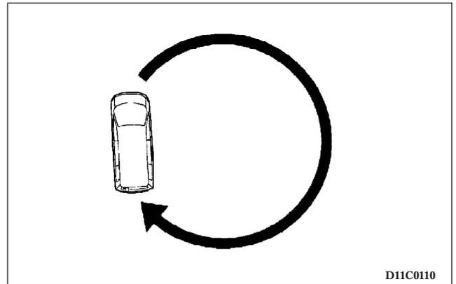
If the “CAL” is displayed, drive the vehicle in a circle at about 5 mph (8km/h) or less until the “CAL” goes off.
