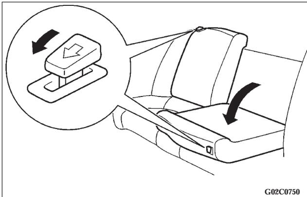
The rear seatbacks can be folded forward to provide additional cargo area. Pull the left and/or right release knobs, and fold the rear seatbacks forward.
