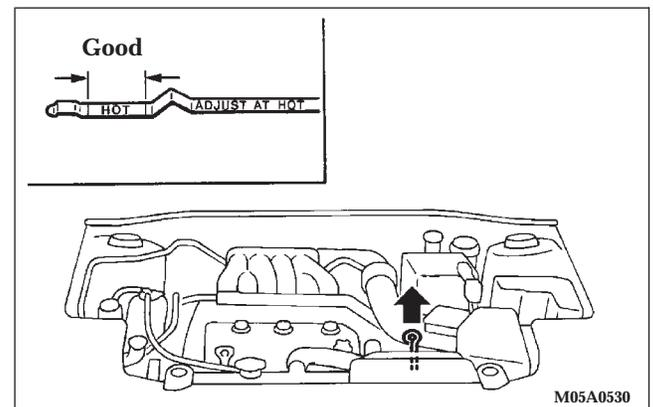
The automatic transaxle should be maintained and serviced by an authorized dealer to obtain the best performance and maximize life. It is important that the transaxle fluid be maintained at the level prescribed.
