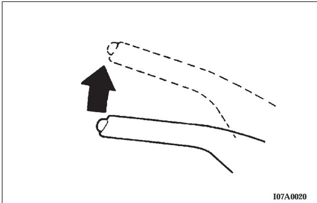
Before leaving the vehicle, make sure that the parking brake is set. To set the parking brake, pull up firmly on the lever. Also place the gear selector in the Park position (automatic transaxle) or Reverse (manual transaxle). To release the parking brake, apply the brake pedal and pull up on the parking brake lever. Push the release button and lower the lever fully.
