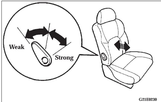
A lumbar support is included in the seatback of the driver's seat. The support has a three position adjustment.
