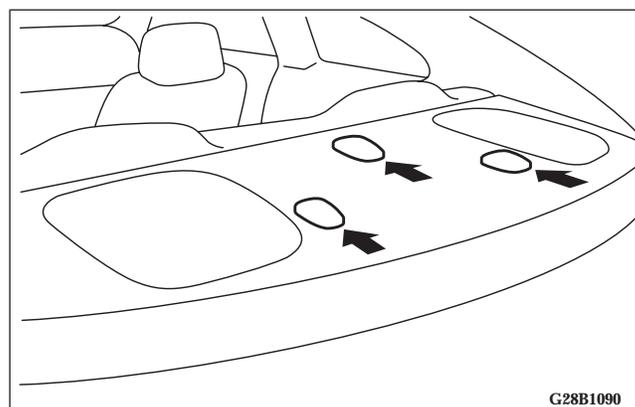
In compliance with the Federal Motor Vehicle Safety Standards, your vehicle has 3 attachment points on the rear shelf, located behind the top of your rear seat. For securing a child seat tether strap to each of the 3 rear seating positions (2 outer and 1 center) in your vehicle.
