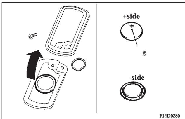
2. Remove the discharged battery from the panic button side of the case half.
