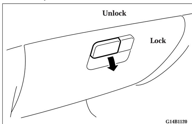
To open the glove compartment, pull the lever.
