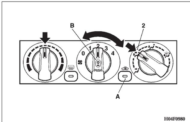
**NOTE:** If the outside air is dusty or otherwise contaminated, or if maximum cooling performance is desired, set air selection switch (A) to the recirculation position and the temperature control dial all the way to the left. Introduce outside air from time to time for proper ventilation.
