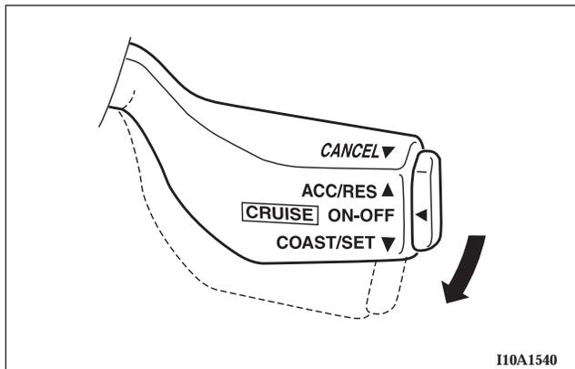
Pull the cruise/speed control lever down and hold it while driving at the set speed, and you will slow down (coast) gradually. When your desired low speed is reached, release the lever.
