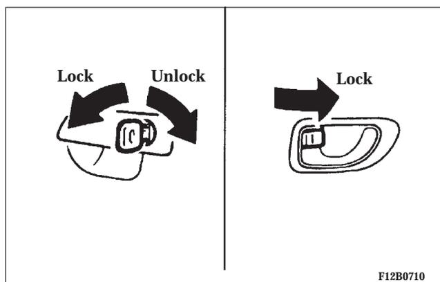
Using the key to lock or unlock the driver's or passenger's (if so equipped) door will automatically lock or unlock all of the doors.
