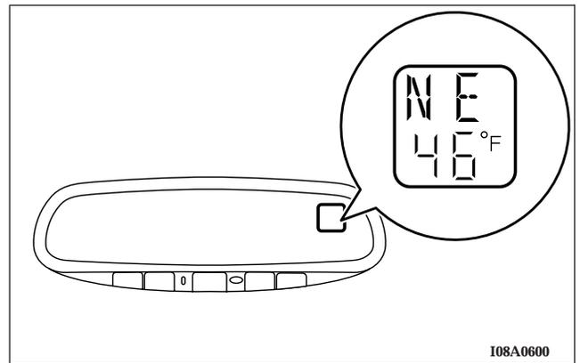
When the ignition key is in the “ACC” or “ON” position, the current outside temperature is displayed.
