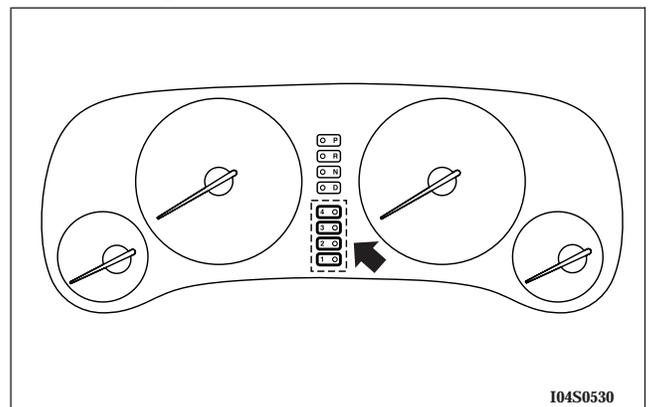
In Autostick, the currently selected gear is indicated by the lights on the instrument panel.
