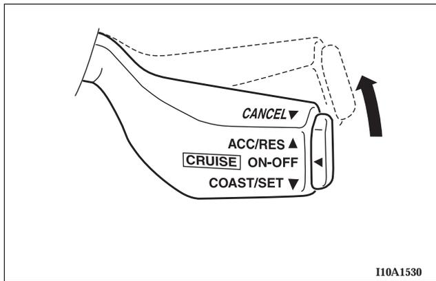
Pull the cruise/speed control lever up and hold it. Your speed will then gradually increase. When you reach your desired speed, release the switch. Your cruising speed is now set.
