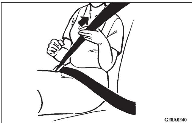
4. Pull up on the shoulder portion of the belt to ensure that there is no slack in the lap belt. The belt will retain the small amount of slack necessary for comfort when you return to your normal seating position. If the belt is still too tight, pull out 6 to 8 inches of webbing, release the belt, and let it return to your chest.
