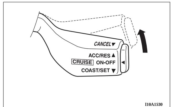
If the speed memory has not been erased, resume the previously set speed by pulling the cruise/speed control lever up while driving at a speed of 25 mph (40km/h) or higher.
