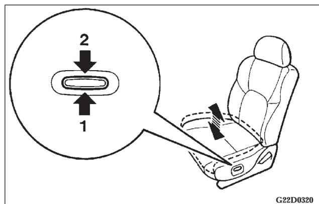
Push the center of the switch to raise or lower the whole seat cushion.
