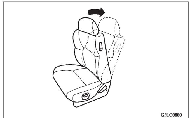
Just by pushing the seatback up into position will lock it in the memorized position.
