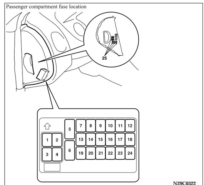
The fuse cover lists the names of the electrical systems and the fuse capacities. Spare fuses are contained in the
