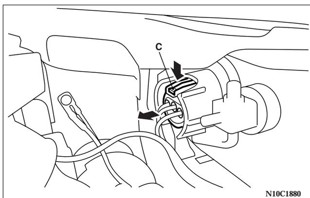
2. Push the connector (C) to disconnect and remove the harness connector.
