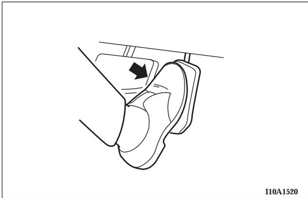
Press the accelerator pedal as you would normally. When you release the pedal, the cruise/speed control will return to your set speed.
