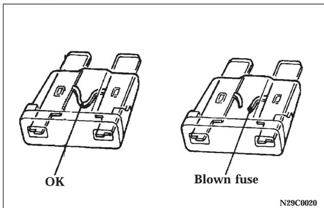
1. Before replacing a fuse, always turn off the electrical item concerned and turn the ignition key to the "LOCK" position.
