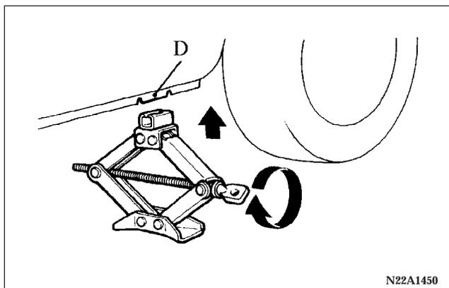
6. Rotate the jack by hand until the flange portion (D) fits in the groove at the top of the jack.
