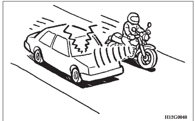
FM can be affected by electrical systems of vehicles in the vicinity, especially those without electronic noise suppression for the ignition system. The disturbance is even greater if the station is weak or poorly tuned.
