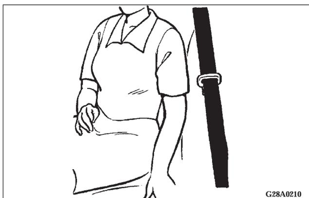
1. Get in the vehicle and sit in a normal correct posture. To reduce the risk of severe or fatal injury caused by an inflating air bag, adjust the driver's seat to the rear most position that still allows you to fully apply the pedals, easily control the steering wheel and safely operate the vehicle. The front passenger should also adjust their seat as far back as possible. Refer to "Supplemental Restraint System (SRS) - air bag" on page 89.
