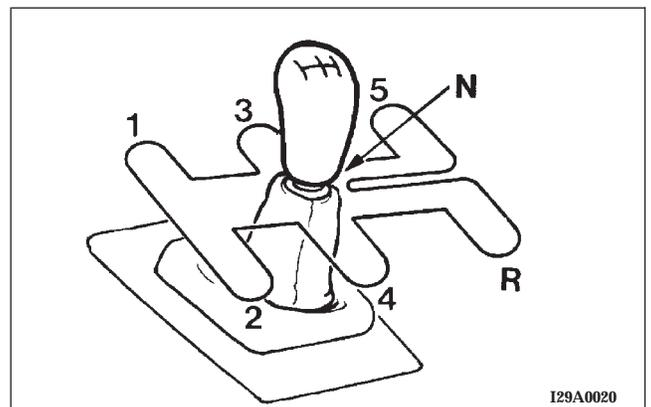
The shift pattern is shown on the gearshift lever. Depress the clutch pedal fully while shifting gears.
