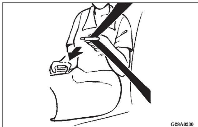
3. Pull the seat belt out slowly while holding the metal tongue. This system will not lock up if you stop or hesitate, so relax and continue to “buckle-up”. Push the metal tongue into the buckle until a “click” is heard. Pull up on the belt to confirm the metal tongue is locked securely in the buckle.
