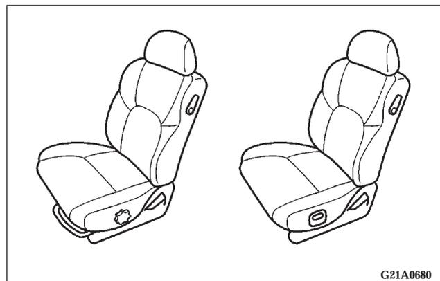
Adjust the driver's seat as far back as possible to a position that enables you to fully apply the pedals, easily control the steering wheel, safely operate the vehicle and also gives you a clear frontal view.
