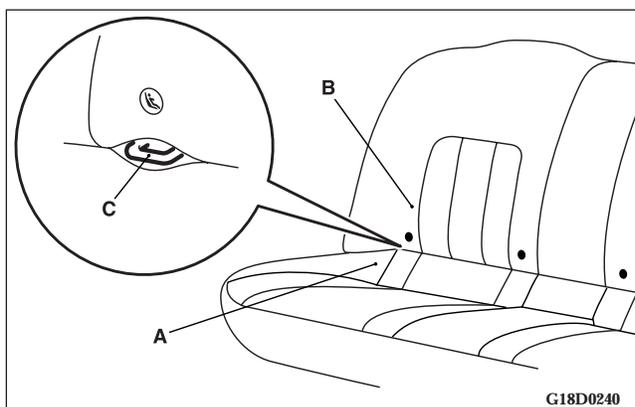
1. Open the gap a little between the seat cushion (A) and the seatback (B) with your hand to locate the lower anchorages (C).
