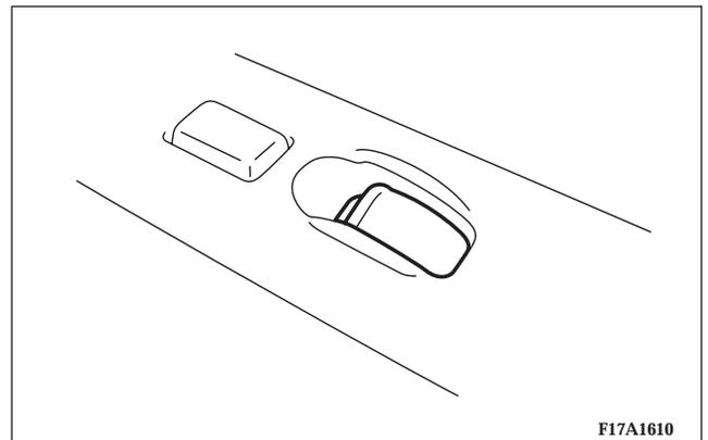
The passenger switch can be used to operate the passenger door window.
