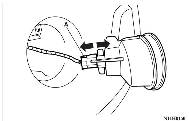
2. Push the connector (A) to disconnect and remove the light bulb.
