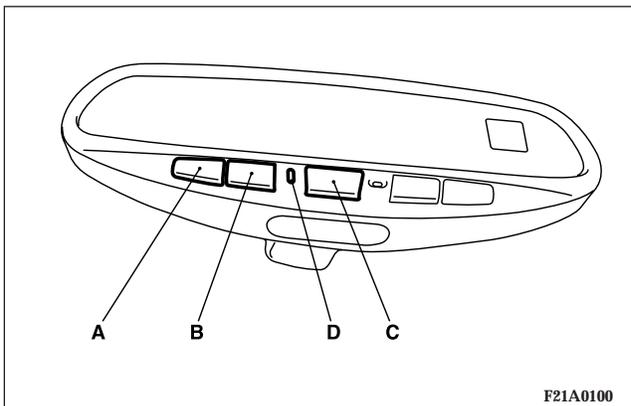
3. Choose one of the three buttons to train. Place the hand held transmitter 1 to 3 inches from the universal transceiver while keeping its indicator light in view.
