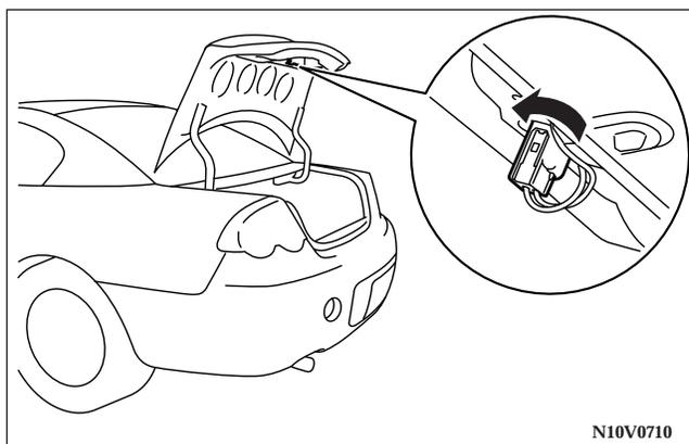
Remove the socket assembly and bulb together by turning it counterclockwise.
