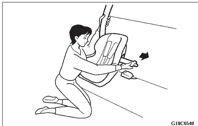
2. Route the unibelt through the child restraint system according to the child restraint system manufacturer's instructions. Then insert the unibelt latch plate into the buckle. Make sure you hear a "click" when you insert the latch plate into the buckle.
