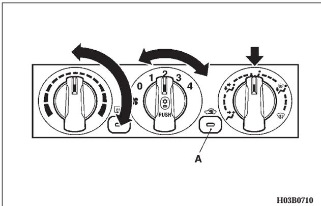
Set the mode selection dial to the position shown in the illustration and set the air selection switch (A) to the “outside” position.
