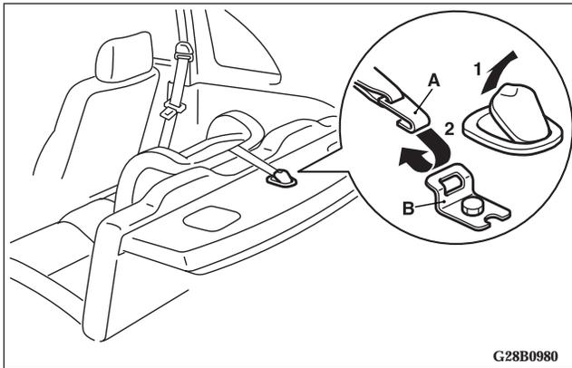
1. Lift the cover from the tether anchor installation point by pulling it back with your hand as illustrated.
