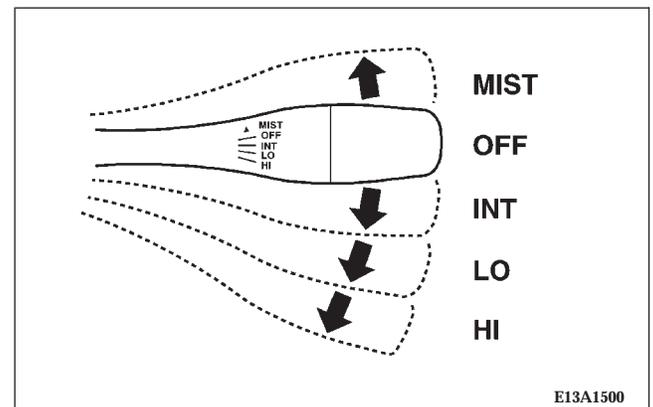
The windshield wipers can be operated when the wiper lever is moved as illustrated above and the ignition key is in the "ON" or "ACC" position.
