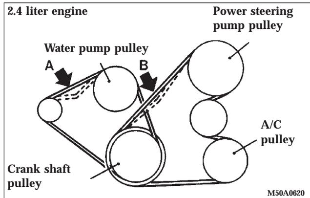
Check the tension of the drive belt. The deflection must be within specifications, when depressed at a point midway between the pulleys as shown in the illustrations with a force of about 100 N (22 lb.).
