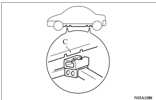
5. Place the jack under one of the jacking points shown in the illustration. Use the jacking point closest to the tire being changed.
