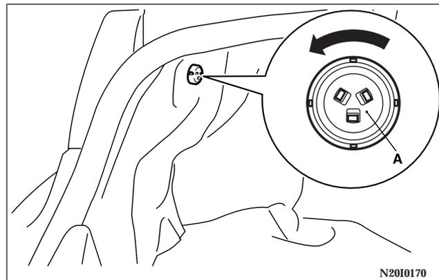
1. Turn the trim cover clip (A) counterclockwise and remove the trim cover clip. Partially remove the trim cover in the trunk.
