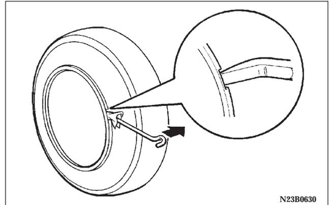
Wrap the tip of the bar with a cloth, insert it deeply into the notch provided in the wheel cover, and pry the cover away from the wheel.
