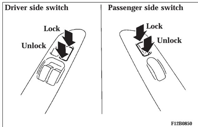
All of the doors can be locked or unlocked by pressing the power door lock switch on the driver's or the passenger's door.
