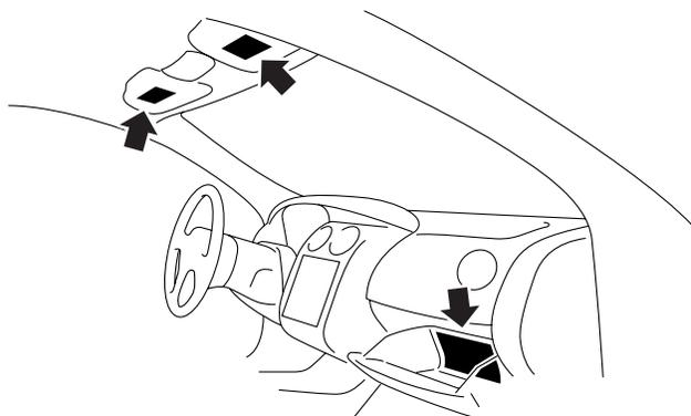
Passenger restraint warning/caution labels for the SRS are located in the vehicle as shown in the illustration.
