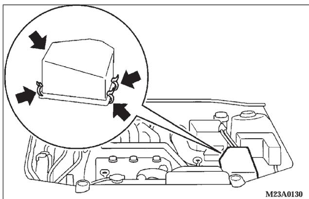
The air cleaner filter will become dirty and loaded with dust during use, and the filtering effect will be substantially reduced. Replace it with a new filter in accordance with the schedule in this manual.
