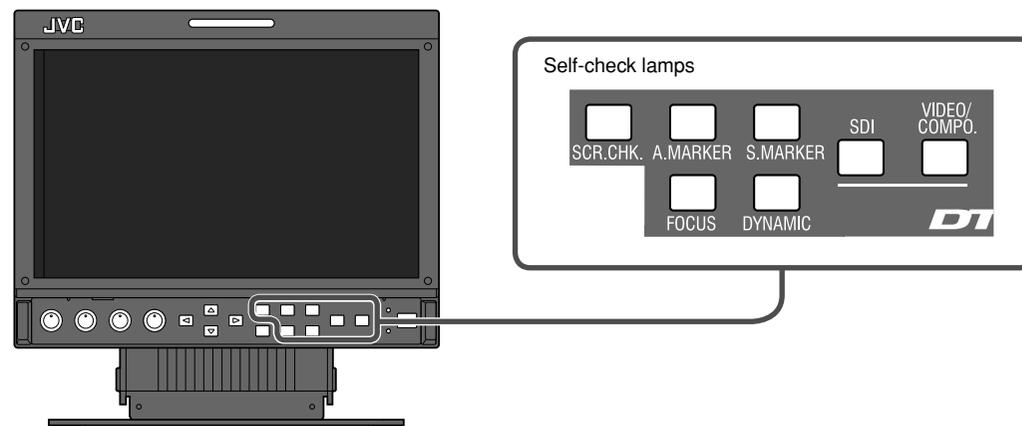
When the screen goes blank and check one or some self-check lamps on the front control panel start flashing...
