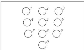
for channel selection and number input in the menus. *To key in two-digit channels (example: 10, 11, 12, etc.), hold the first digit key down to call the placeholder dash on the display (I-), then enter the second digit.*
