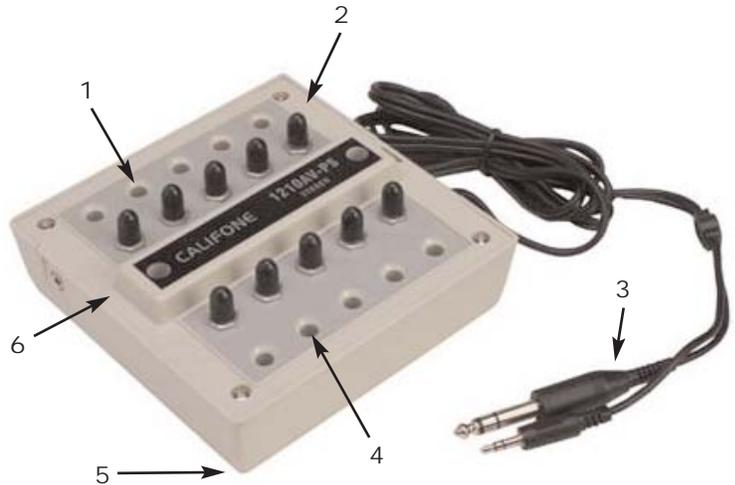
The key to listening centers is the jackbox, the distribution point to the headphones. *Califone* gives more attention to this stereo jackbox with silver-plated contact points for a solid connection and moisture resistance, individual volume controls, rugged ABS plastic housing for durability, 1/4" and 3.5mm plugs.
