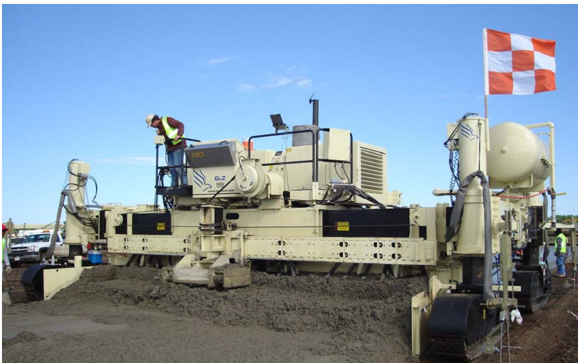
Figure 24. Spreader (plow) at the front of a paver.
