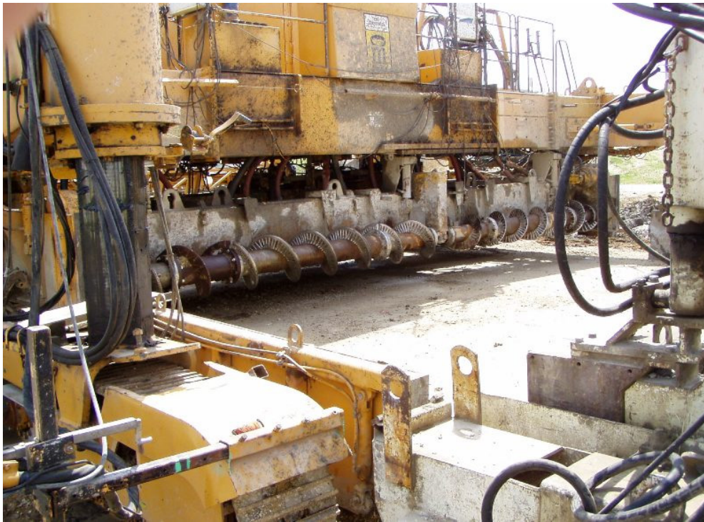
Figure 23. Auger located at the front of a paver.
