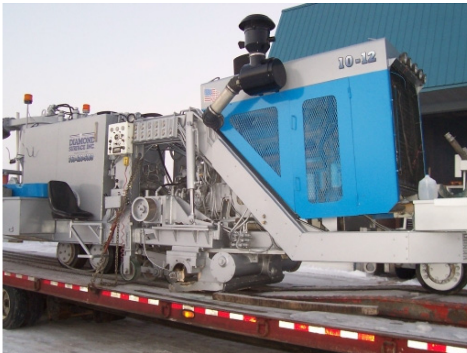
Figure 2. Grinder used for large-scale concrete pavement texturing operations.
