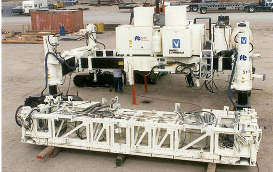
Figure 20. Paving kit for a slipform paver.
