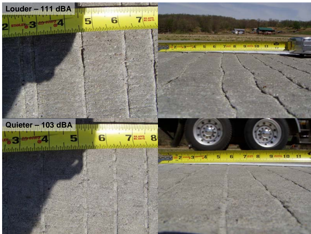
Figure 11. Variability of transverse tined surface and its effect on OBSI noise level.
