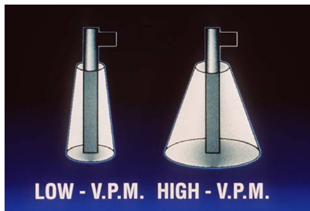
Figure 26. A difference in vibrator frequency will influence the volume of concrete that is consolidated.
