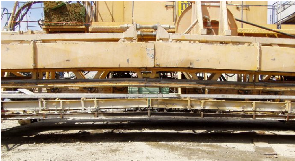
Figure 27. Forming pan set for a crowned pavement.
