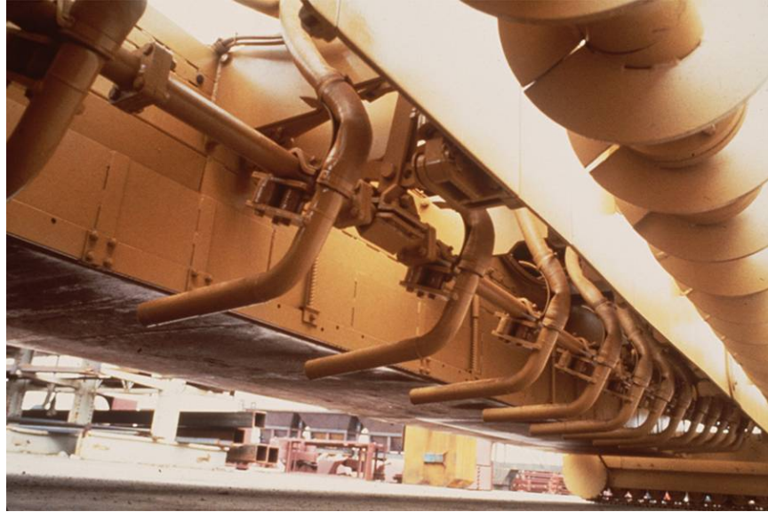
Figure 25. This photo shows a typical line of vibrators mounted to the paver.
