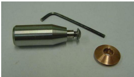
Ready the Adapter Shaft and screw, and the wrench. Remove the screw and set it to the side for a moment...
