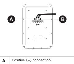
3. Connect the negative and positive speaker wires from the speaker to the corresponding terminals on the amplifier.
