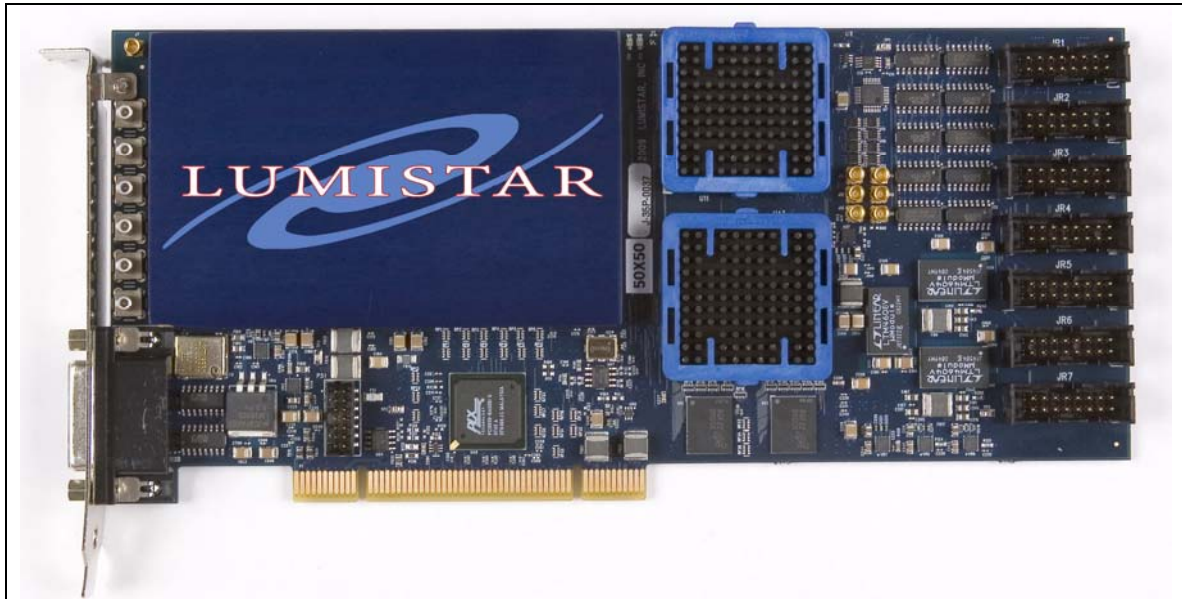
Figure 1-20 LS-35 Dual Channel Multi-Mode Demodulator CCA
