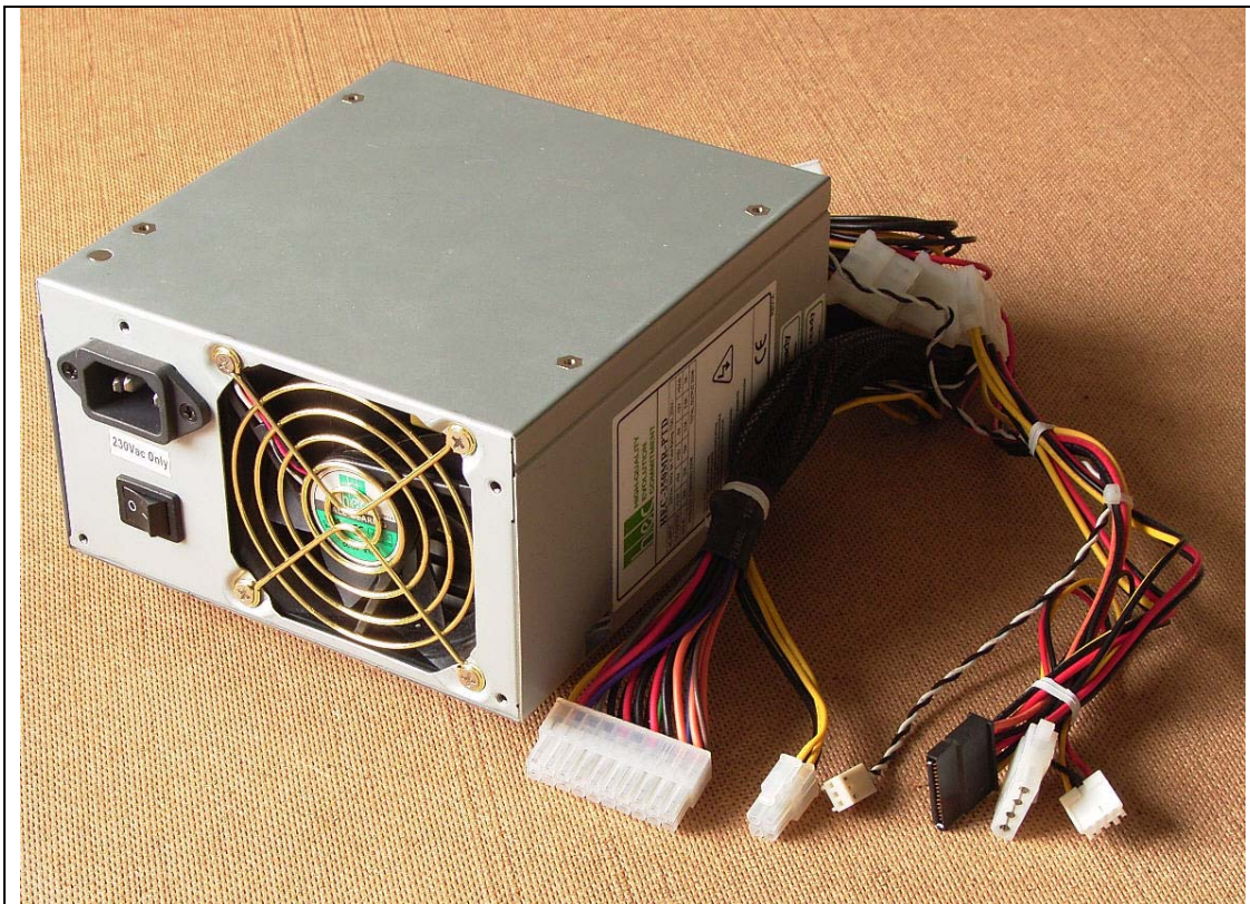
Figure 1-6 a typical ATX style System Power Supply used in the LS-28
