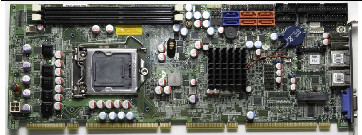
Figure 1-9 a typical SBC used in the LS-28-QRS & -R2D3
