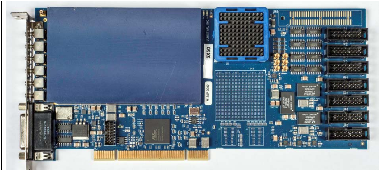
Figure 1-23 LS-34 Single Channel Multi-Mode Demodulator CCA
