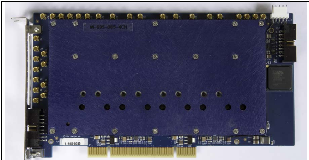
Figure 1-15 LS-69-S I/O Routing CCA
