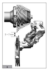
If the distance is too large, tighten the screw G (Fig. 4), if the distance is too short, unscrew the screw.
