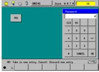
(3) Input the password and press [OK], and the operating panel closes.
