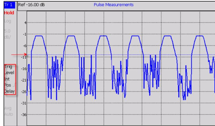
Trig Level = -10 dBm, Trig Type (**Int**), Pos Slope (/), Delay
