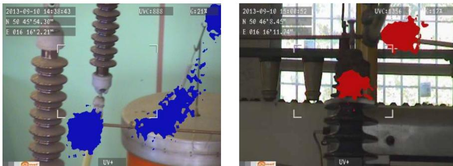
Fig. 3, 4. Corona discharge in laboratory conditions.
