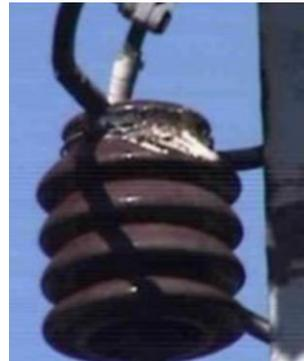
*Fig. 9, 10. Corona discharge and its effects.*
