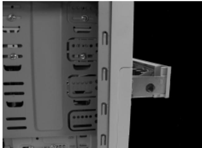
6. Attach the other end of the cable and install the PCIU5 into a PCI slot, following the instructions described at step 4 to 5 in Chapter 3-1.
