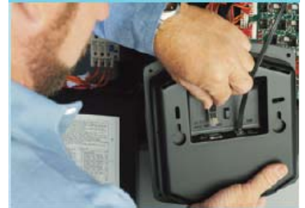
Removable display makes troubleshooting servicing easier.
