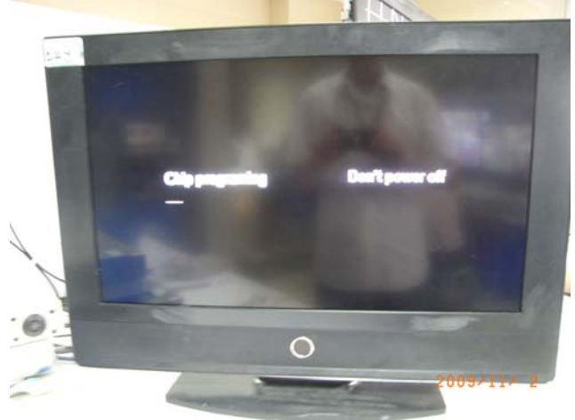
20. After 20 sec. Led is flash very fast. display Chip programming.
