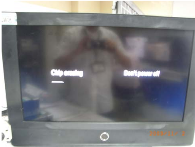
19. After 10 sec. Led is flash slowly, display Chip erasing.
