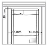
Install the drver far from gas ranges, stoves, radiators or hobs as flames may damage it. If the dryer is installed below a worktop. ensure there are 10 mm between the upper panel of the dryer and any objects above it and 15 mm between the sides of the machine
