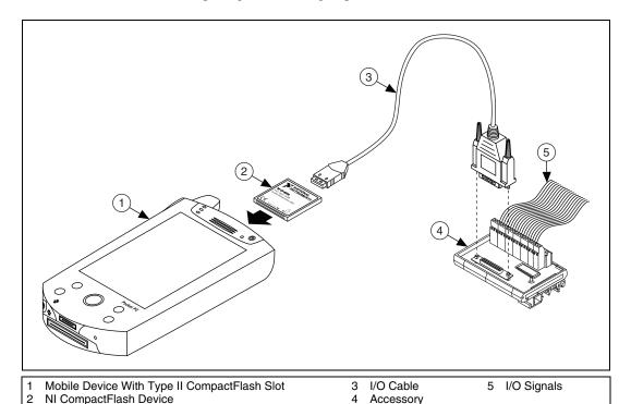
NI CompactFlash devices have two connectors: a 50-pin CompactFlash bus connector on one end, and an I/O connector on the other. The NI CompactFlash device is keyed so that you can insert it only one way. Insert the NI CompactFlash device in the slot until the connector is firmly seated.
