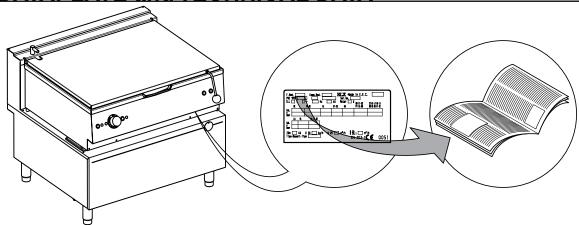
**ATTENTION** This manual contains instructions relevant to various appliances. See the dataplate located under the control panel to identify the appliance (see fig. above).
