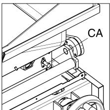
• To replace the detection electrode, remove the left side, loosen the fixing screws and remove the components.
