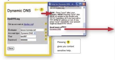
A dynamic DNS client allows your servers to be accessed by an Internet name (URL) instead of an IP number, even if you have not received a fixed IP address from your operator. It is very useful if you want to operate a WEB server or when using the IX66 as a SIP server.
