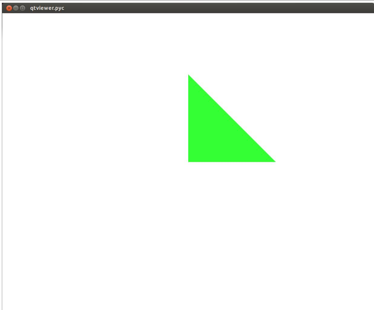
If you pass 6 vertices/normals/colors, it will display 2 triangles and so on. As a sidenote, it is very efficient and in fact `chemlab.graphics.renderers.TriangleRenderer` is used as a backend for a lot of other renderers such as `SphereRenderer` and `CylinderRenderer`. If you can reduce a shape in triangles, you can easily write a renderer for it.
