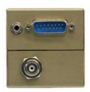
The XCOM VHF 760 Transceiver has a 2.25" (57mm) face for fitting in a normal aircraft small instrument hole. The case is 5.1" (129mm) long, 2.4" (61mm) wide and 2.4" (61mm) high. The unit is secured to the aircraft dashboard by 4 screws and is self supporting, requiring no additional supports, trays or brackets.
