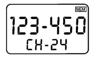
The display will show the frequency being entered and the first free memory channel. If all memory channels are occupied, then channel 1 will be selected and the currently stored frequency will be shown. Press **MEM** again to overwrite the current frequency with the newly entered frequency.
