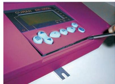
Detach the keyboard / display unit carefully by prying it with a screwdriver.
