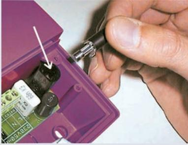
Switch off the voltage from the regul. Press the fuse socket and turn it counter clockwise. Change the 160mA (5x20mm) glass tube fuse. Press and turn the fuse socket clockwise into place.
