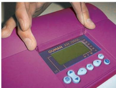
Remove the clear cover. Press as illustrated in the picture and pull the cover out of place.
