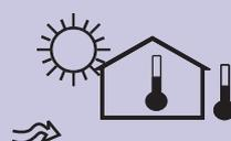
Supply water regulation according to the outdoor temperature, including the inside temperature measurement (room compensation) and both sun and wind compensation.
