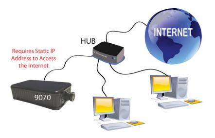
In this case, the 9070-Lite is being connected to the internet through a hub, which is different from a router. The hub does not provide DHCP, and therefore would require that this setup have a static IP Address that is provided by the ISP.
