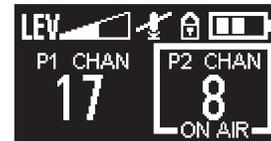
5. Push the Menu button and note that either “P1” or “P2” shows up on the top left corner of the screen. This indicates which Preset you are adjusting.
