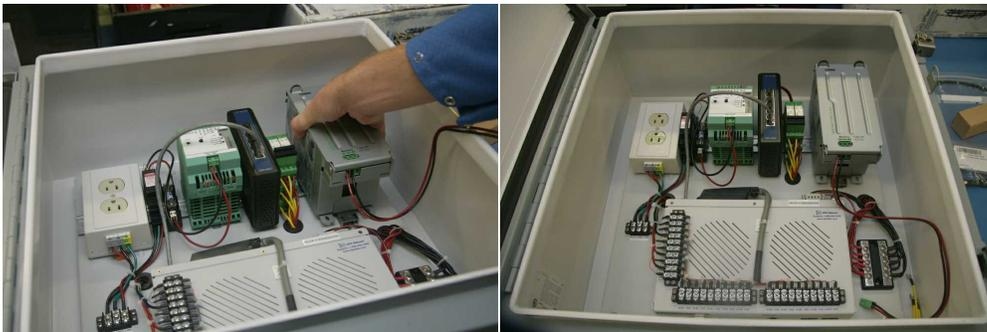
3. To remove the battery simply place a screwdriver into the tab. Gently pull the tab back while lifting the battery.
