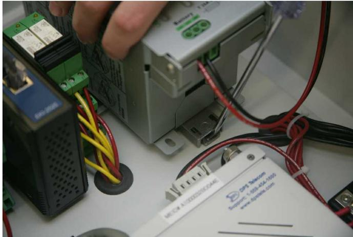
4. Locate the input inside of the casing (circled in the second image below). Attach the power wires from the battery to the input.
