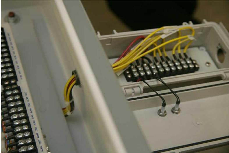
2. Match the wire label to the silk screen, terminating each wire on the right terminal. The top 4 terminals are the 2 LEDs (warning and interrupt). The lower 6 are the 2 relays (warning and interrupt).
