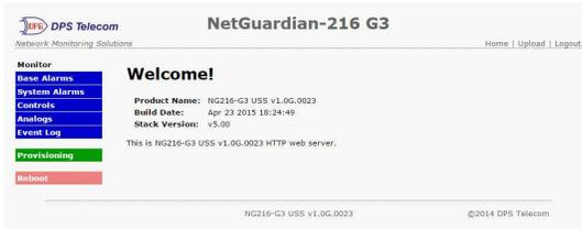
The Utility Shutdown System features a built-in Web Browser Interface that allows you to manage alarms and configure the unit through the Internet or your Intranet. You can quickly set up alarm point descriptions, view alarm status, issue controls, and configure paging information, and more using most commonly used browsers.
