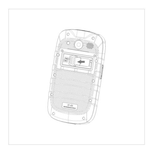
5.Insert the battery cover: Insert the back cover and rotate two screws clockwise to lock the back cover.
