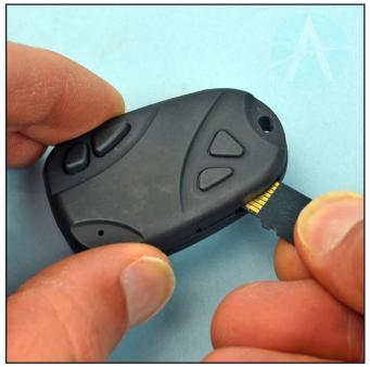
Insert the Micro SD card with the metal contacts facing upward.
