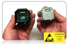
Disassembling the module can cause permanent damage and will void the warranty. Operating the module outside of the specified input voltage range or the specified operating temperature range can cause permanent damage and coud also damage the TAU2 core. The module front is not sealed. Avoid exposure to dust and moisture. This module contains electrostatic-discharge-sensitive electronics and should be handled appropriately.
