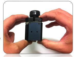
2. Plug module directly into the rear of the camera. There is a white 50-pin connector that will mate. I tis recommended slowly and carefully insert the camera into the module and subsequently keep the whole system in to the both hands such as on the picture. Afterwards you should push to the module and camera. Workswell company is not liable for any damage of camera caused by wrong insertion into the module .
