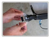
Returning to the wingtips, detach the lines from the tips of the bladders and carefully fold the bladders tips up into the ends of the wingtip sleeve. Carefully fold over the end cap and securely fasten the Velcro pieces together ensuring the bladder cannot poke out once inflated.
