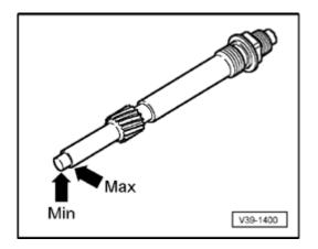
Oil level must be between min.- and max.- marking.
