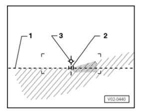
With the low beam switched on, check whether the horizontal light-dark border contacts the hyphenated line - 1 - of the test surface and
