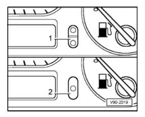
One button - 2 - is allocated below the clock at right for setting the time.
