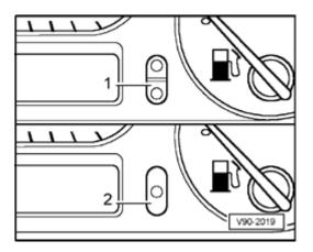
Two press buttons - 1 - are located below the tachometer at right for setting the clock. The hour is set using the upper button - h - , the minute is set with the lower (min).
