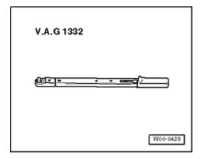
Torque wrench V.A.G 1332 (40 -200 Nm)
