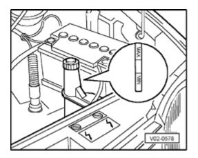
Fluid level must be between min. and max. marking.
