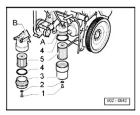
There are two different versions of the oil filter -  ${\bf A}$  - and -  ${\bf B}$  -
