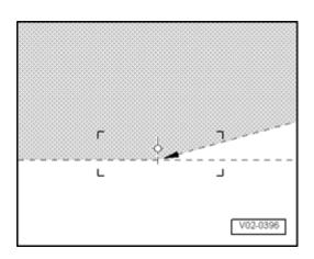
For the previous test screen with 15° -setting line, adjust as for new test screen. But to avoid incorrect settings ignore 15° -setting line.
