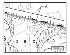
For these engines, if damage to toothed belt due to lateral scouring at toothed belt guard is detected, especially damage illustrated in figures - B - and/or - C - , perform the following repair measure:
