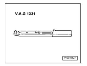
Torque wrench V.A.G 1331 (5 - 50 Nm)
