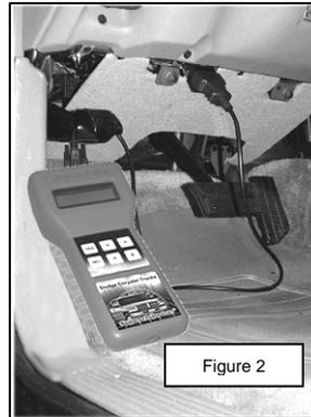
Insure the ignition switch is OFF, then press the '>' key on the keypad. The MAX MicroTuner displays the following messages:
