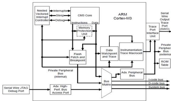
Fig 2. Block Diagram of ARM Cortex M-3 Processor Core
