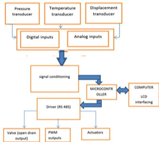
Fig 3. Electronic Module for Hydraulic Damper Test Bench using SOC
