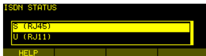
ISDN physical interface selection detail
