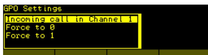
GPOs operation mode configuration submenu
