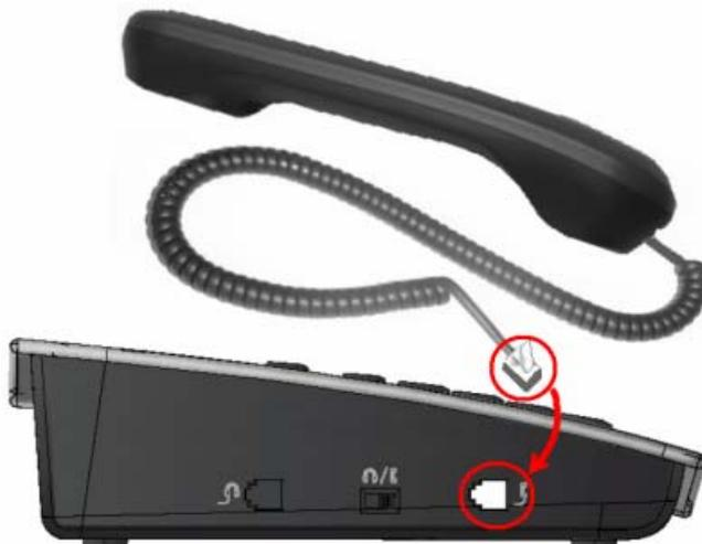
Figure 1.2 Connect the handset to the IP phone base unit
