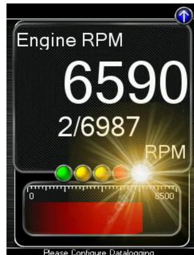
Press **[OK]** and using the **[Up]** and **[Down]** buttons, set the RPM to the desired level to have the shift light flash. Press **[OK]** to save the RPM you have selected. By default, the shift light RPM is set above the stock redline. This essentially disables the shift light since that RPM will not be reached. You will need to lower the shift light RPM to enable this feature.
