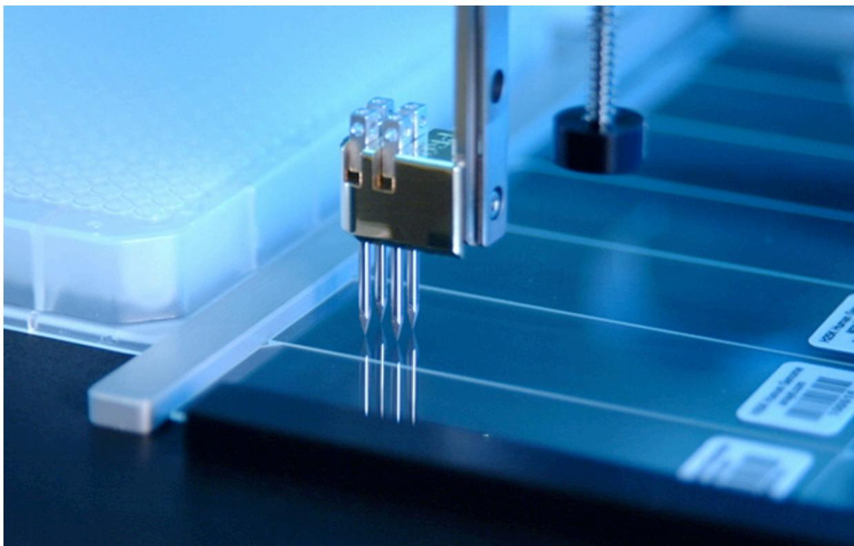
**Figure 12.** SpotBot® 3 Personal Microarrayer Professional Series Printhead and four 946MP4 Microarray Printing Pins shown in the printing position on the deck. An “overtravel” of 0.5 mm is used to ensure precise printing onto each glass substrate slide. The SpotBot® 3 Protein Edition Microarrayer preserves the activity and integrity of printed samples by cooling the entire deck, including the microplate samples and substrate slides.
