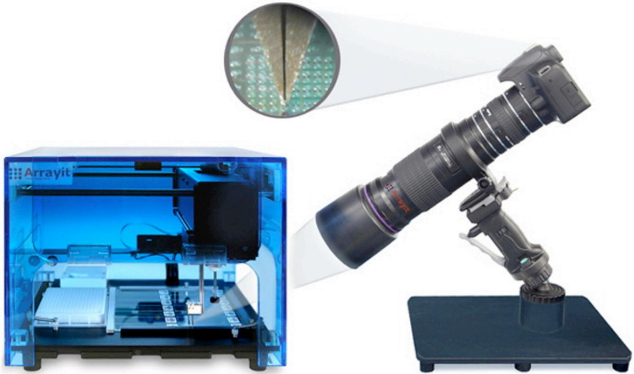
**Figure 15.** SpotBot® 3 Personal Microarrayer Vision System with high-resolution digital camera, tripod, and custom software interface to view and record absolute positional coordinates on the printing deck. The Vision System allows visualization of microscopic substrate elements such as 100  $\mu\text{m}$  microelectrodes (see insert) using a digital camera with 10  $\mu\text{m}$  spatial resolution. Highly recommended for aerospace, bio-engineering, material science applications.
