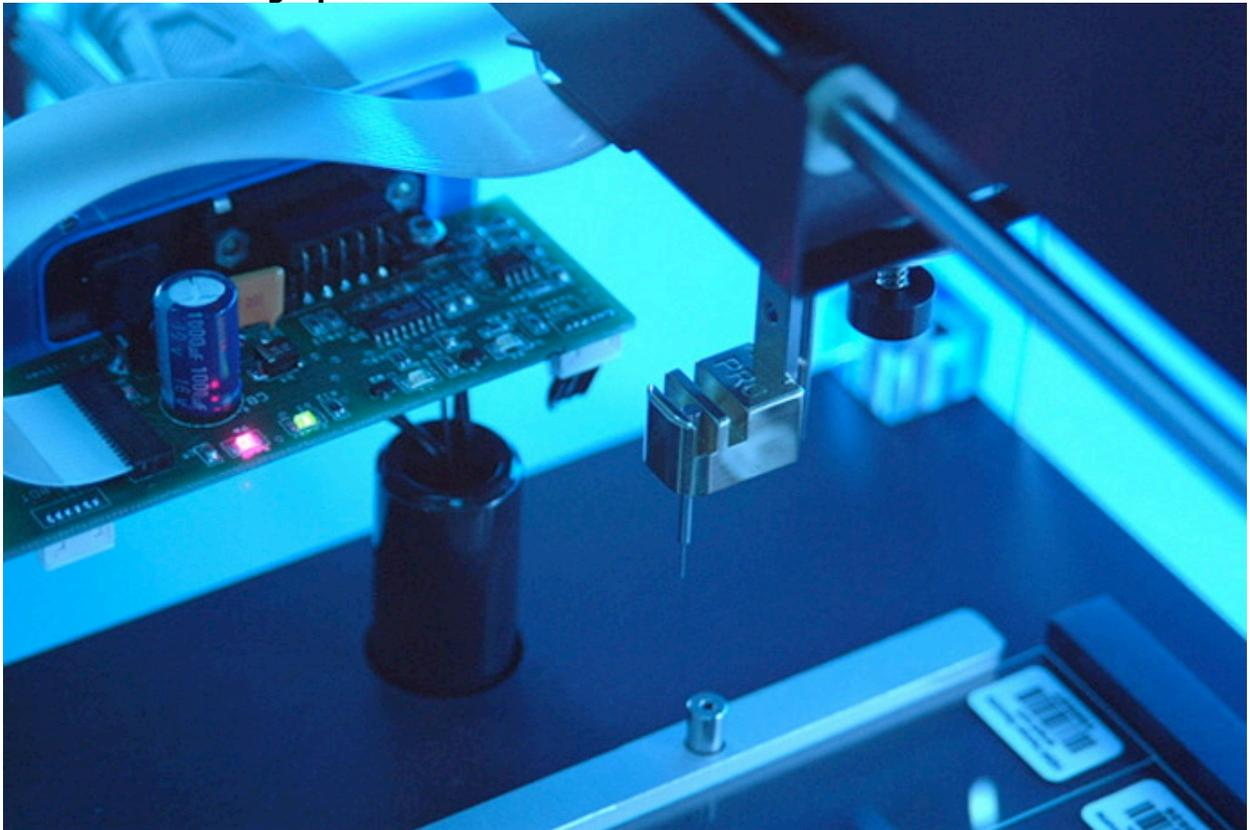
**Figure 1.** SpotBot® 3 Microarrayer in the “home” position. The printed circuit board and operation lights (top left) permit fully automated computer-control. The professional printhead (center) contains a calibration pin in the first of 4 pin apertures.
