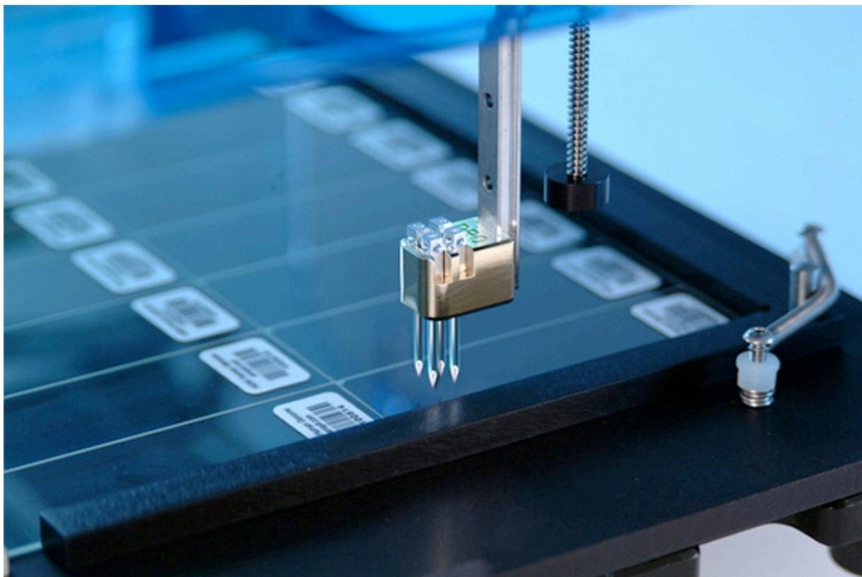
**Figure 14.** SpotBot® 3 Personal Microarrayer Professional Series Printhead and 946MP4 Printing Pins in the "safe Z" position over the glass substrate slides. The spring-loaded L-Bracket immobilizes the substrate slides on the platen during printing to maintain a high degree of positional precision and accuracy.
