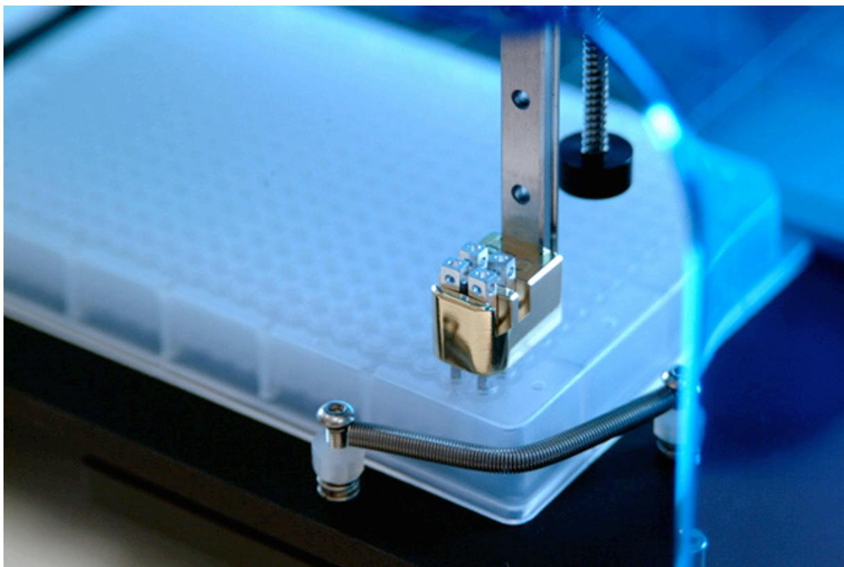
**Figure 3.** SpotBot® 3 Microarrayer in the sample loading position. The Professional Series Printhead and 4 946MP4 Pins move into the loading position in the first group of 4 wells in the 384-well microplate. A loading time of 3 seconds allows each pin tip to load 0.2  $\mu$ l of sample from each well containing 5  $\mu$ l of total sample volume.
