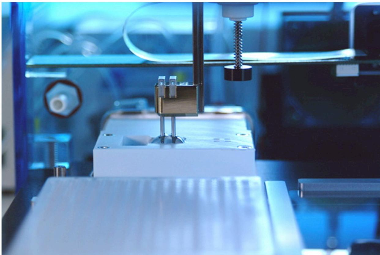
**Figure 2.** Megasonic Wash Station on the SpotBot® 3 Protein Edition Microarrayer. Megasonic waves propagated through the wash buffer facilitate highly efficient pin cleaning. The dry port to the right of the wash station uses pressurized air to dry the pins after cleaning.
