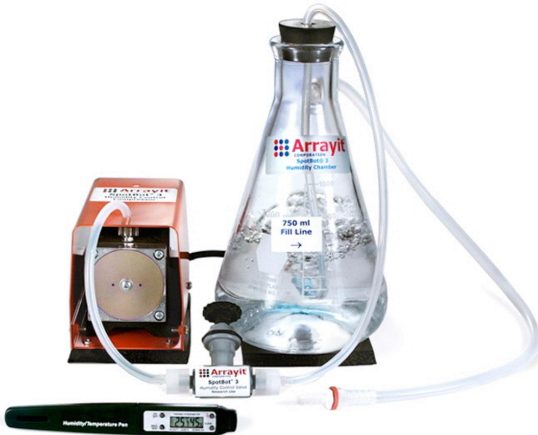
**Figure 5.** The Humidification System for SpotBot® 3 Personal Microarrayers includes a Humidity Control Compressor, Control Valve, Humidity Chamber, and Temperature and Humidity Pen. The system allows humidification of the internal instrument chamber from ambient to 80% relative humidity (RH) with an accuracy of  $\pm 1\%$ . The same core components and instrument port are used for the Dehumidification Apparatus (see Fig. 9).
