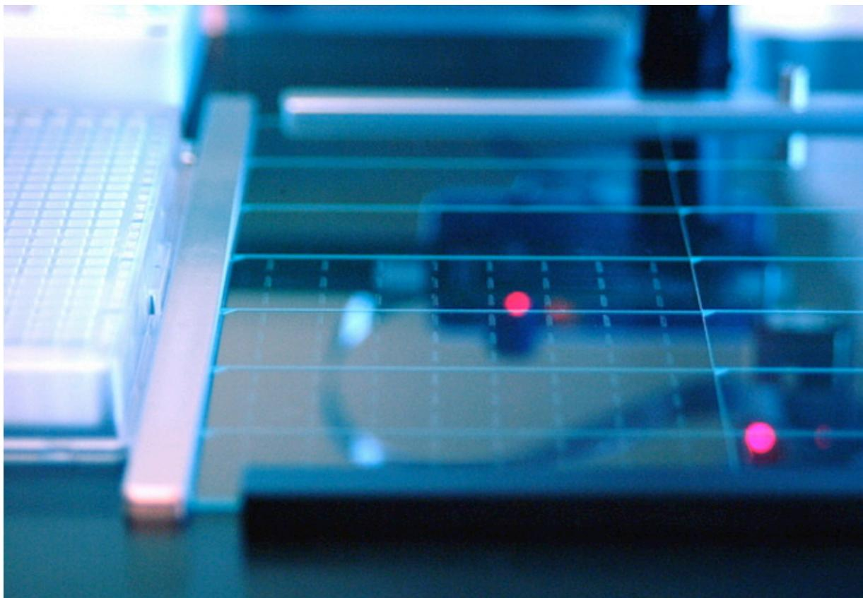
**Figure 6.** Multiple microarrays per substrate printed with a SpotBot® 3 Personal Microarray Robot. Shown is a photograph of the SpotBot® 3 platen containing [SuperAmine Microarray Substrates](#) printed with a SpotBot® 3 Personal Microarrayer running [946MP4 Pins](#) printing at 175  $\mu\text{m}$  spacing. A total of 24 microarrays per substrate were printed using the Multiple Microarray Format SpoCLE Generator version 1.1.02, which can be downloaded at <http://spotsupport.com>.
