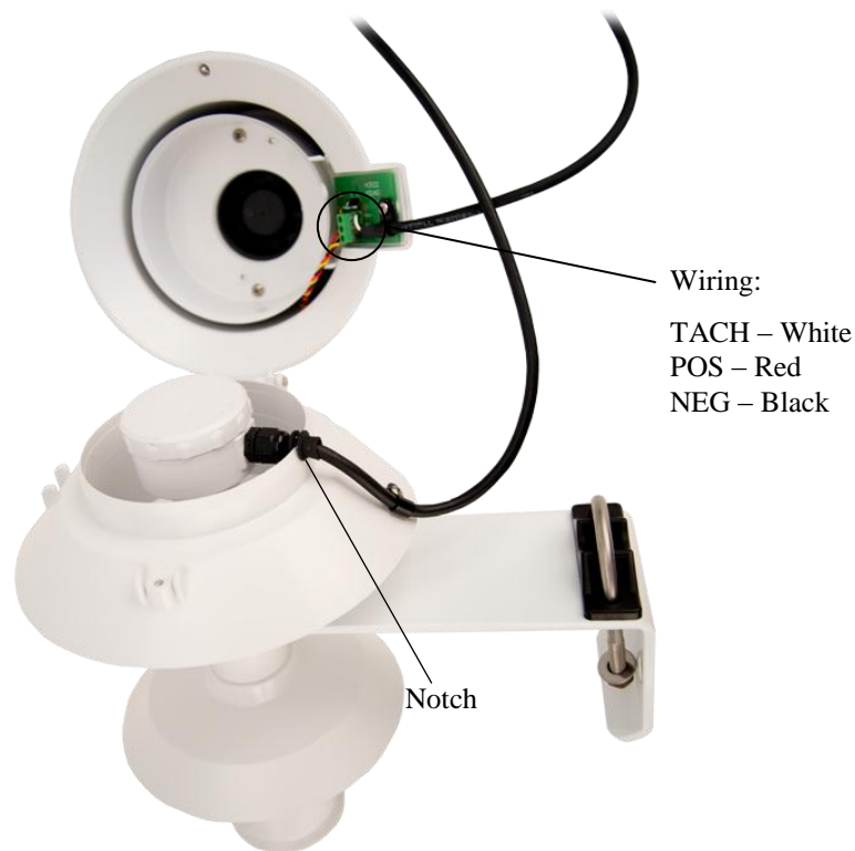
Figure 7-4. 43347 probe mounted inside the 43502 shield
