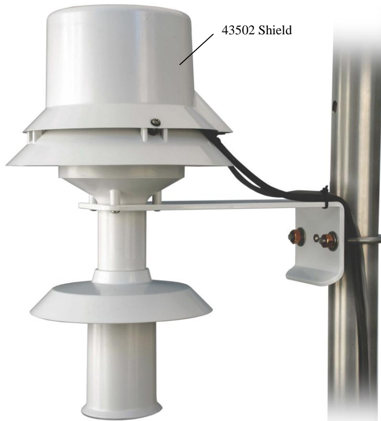
Figure 7-1. 43502 Radiation Shield mounted to tripod mast
