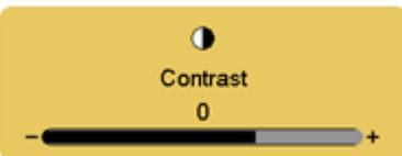
Press the Brightness / Contrast button twice to display the Contrast control. Press the ◀ or ▶ button to adjust the contrast. Setting the contrast too high or too low causes loss of some grayscales. Color saturation may appear incorrect.
