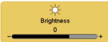
Press the Brightness / Contrast button to display the Brightness control. Press the ◀ or ▶ button to increase or decrease brightness. Setting the brightness too high or too low will decrease the amount of visible grayscales.
