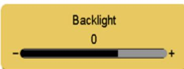
Press the Brightness / Contrast button three times to display the Backlight control. Press the ◀ or ▶ button to set the backlighting.
