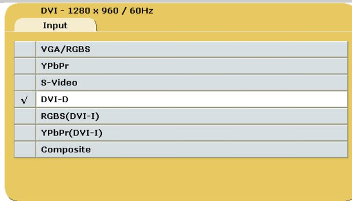
When the display is powered on and **Auto Source Select** is **on**, then **Auto Source Select** looks at the previously selected input first. If a signal is present it is displayed, otherwise **Auto Source Select** starts scanning the inputs for a signal. When the display is powered on and **Auto Source Select** is **off**, the previously selected input is the only input that the display looks at.
