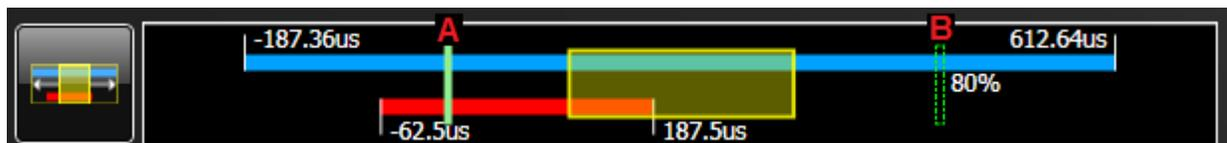
The **WorldView** is primarily a high-level presentation of the current relationship between your displayed acquisition(s) and your current view in the main waveforms display.
