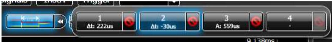
When the **Cursor** tool is enabled, you are currently armed with the selected cursor pair on the waveform display. When expanded, the tool's detailed control provides storage for up to 4 cursor pairs. When cursors are placed on the display, they are highlighted when the pair is selected from the numbered cursor pair. Remove a pair by clicking the **Remove Cursor** button on the right side of the numbered cursor pair.
