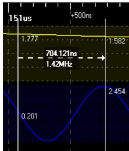
The following screenshot shows a cursor pair placed on the waveforms display.
