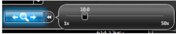
Enable the magnifier tool at any time by clicking the main portion of the control. Now, move your mouse anywhere over the waveform display and an additional, time-magnified display is drawn inside a boxed, magnified area. Use the slider control or mousewheel to adjust the magnification factor inside the time-magnified display. The slider bar updates along with your mousewheel adjustments.
