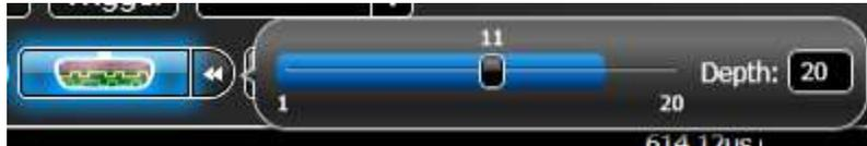
**RearView** keeps a history of the last **N** acquisitions. View your stored acquisitions by setting your trigger to **Stop** and using the slider on the detailed control to flip through the history. The currently selected acquisition is shown in the waveform display area.
