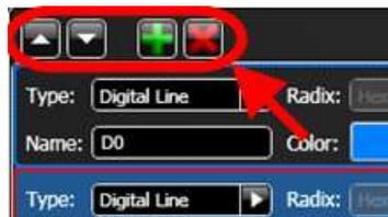
**Note:** Making any modifications to the Signals List or the Signal Setup in any way (even adding new signals) immediately affects currently displayed acquisition data on the Waveform Display Area without requiring a refresh from the device(s).
