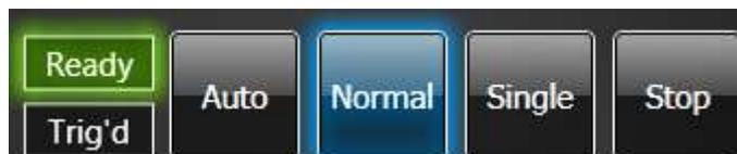
The modes **Auto**, **Normal**, **Single**, and **Stop** behave similarly to an oscilloscope.
