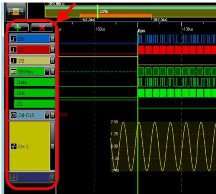
**Note:** Signals contain icons indicating the waveform type they are configured to display.
