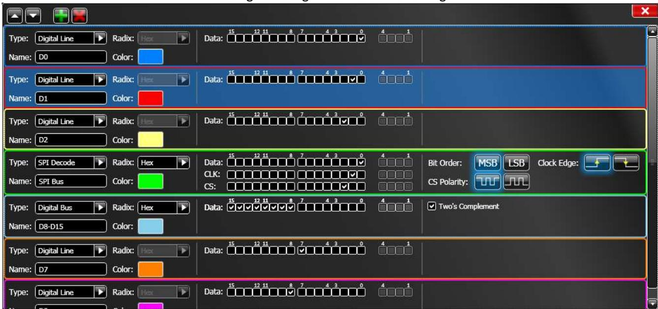
The Signals list allows you to conveniently configure all the signals at the same time. Each row represents a single signal. Inside a single row, you can modify the signal **Type**, **Name**, **Color**, and **Source Channel(s)**, along with additional options depending on the signal **Type** selected.
