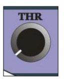
The sound THRESHOLD is used to ground balance the detector. Slowly turn the THRESHOLD knob to the right until you hear just one or two ticks per second.
