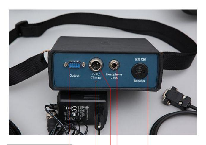
Serial data logging and imaging port is used to transfare scans to logger for the use of 3-D imaging software
