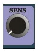
On the Front Panel is the SENSITIVITY knob. The sensitivity level alters how responsive the detector is to signals received from the search coil. The higher the sensitivity level is set the more responsive the detector is.
