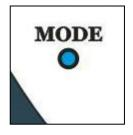
On the Front Panel is the Blue LED indicator. During the DELAY controls adjustments OR when you press the RESET button, this LED indicates that you are in MODE selection.
