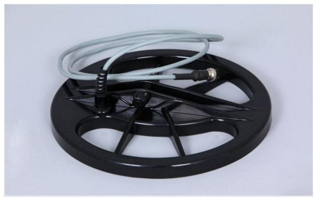
An alternative search coil for Megapulse SR 126 is the CABLE COIL with size 2/2 m. This search coil offers FIVE more ARANGEMENTS to suit your search needs. This search coil can be arranged as 0,50/0,50; 1/1 m; 1/3 m and 2/2m coils by fastening the windings on free frame (from PVC for example) with tape. It can also be arranged in form as "eight".
