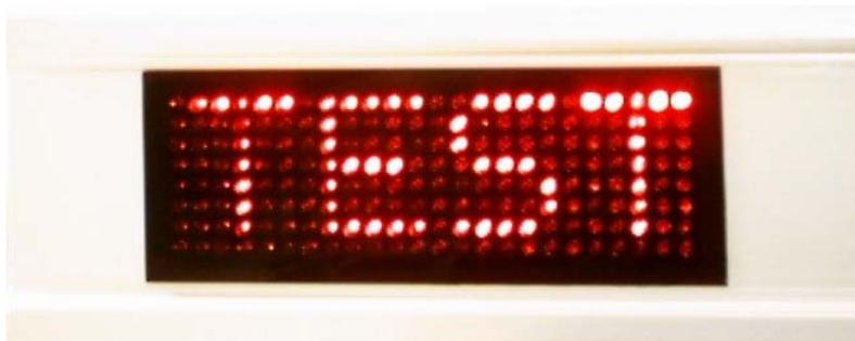
Figure: LED-Matrix Display, short version
