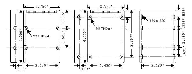
These drawings are meant to provide some guidance, but you must confirm these against a drive in hand or the drive manufacturers specifications before beginning your mechanical design.
